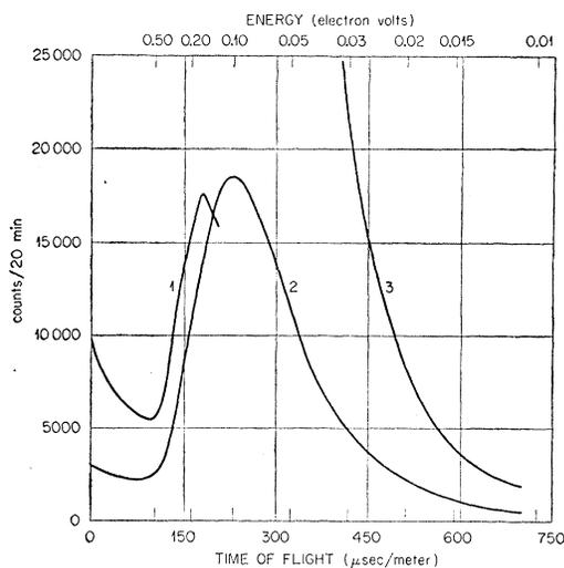
FIG. 1. Typical counting rate curves of the time-of-flight spectrometer for several channel widths and rotor speeds. The data for Curve 1 were taken with 2.45  $\mu\text{sec}/\text{meter}$  channel width and 2.02  $\mu\text{sec}/\text{meter}$  burst width, resolution width 3.3  $\mu\text{sec}/\text{meter}$ . Curves 2 and 3 were obtained with 8.42  $\mu\text{sec}/\text{meter}$  channel width and 5.97  $\mu\text{sec}/\text{meter}$  burst, resolution width 10.2  $\mu\text{sec}/\text{meter}$ .
