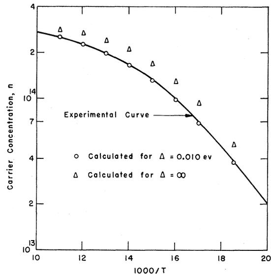
FIG. 2. Experimental carrier concentration vs temperature curve for sample SP1A, and points calculated from Eq. (1) for  $\Delta = 0.010$  eV and for  $\Delta = \infty$ .
