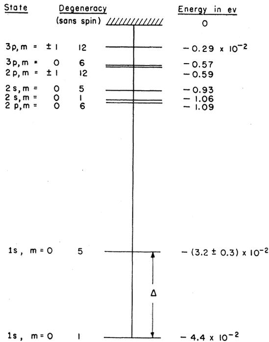
FIG. 1. Theoretical energy level spectrum for a phosphorus donor impurity in silicon (after Kohn and Luttinger).
