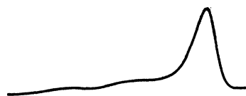
FIG. 4. Glow curve of NaCl recorded by a 1P21 photomultiplier through a 5-mm thick sheet of glass, showing that the first peak has been practically suppressed.
