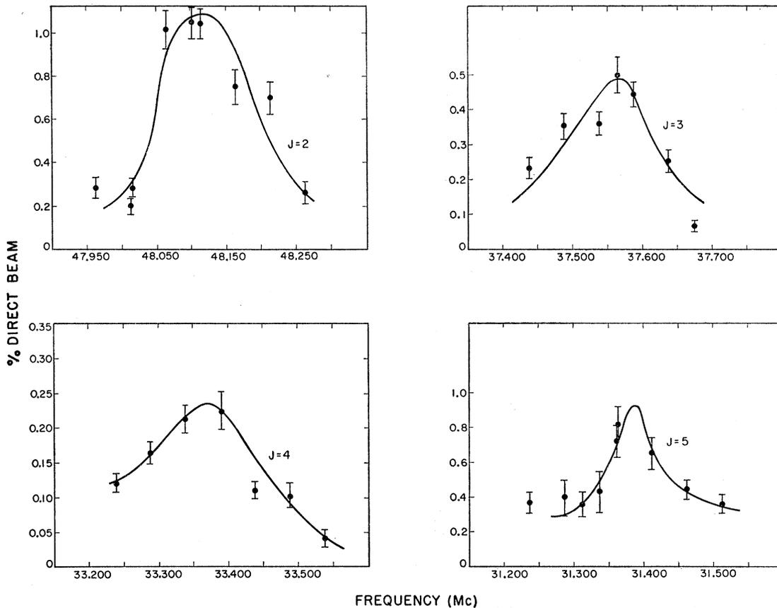
FIG. 1. Transitions in the four observable states of  $\text{Cm}^{242}$  at 13.4 gauss.
