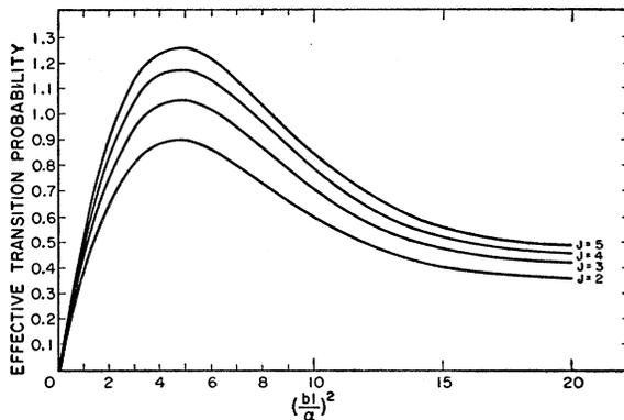
FIG. 3. Calculated transition probabilities for the four states of curium. The abscissa is a quantity which is proportional to the square of the applied rf current. The ordinate is the sum over all flop-in transitions in the particular  $J$  state, of the Majorana transition probabilities averaged over the atomic-beam velocity distribution.
