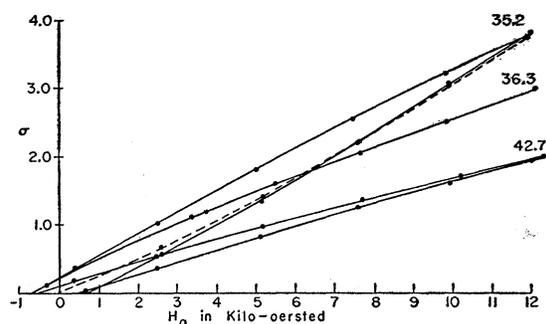
FIG. 6. Magnetization as a function of applied field at 4.2°K. The curve for 36.3 atomic percent aluminum is the demagnetizing portion of a hysteresis loop. The whole loop is shown for the other compositions. The dotted curve is the initial magnetization curve after cooling to 4.2°K in zero field.
