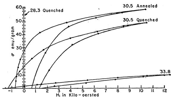
FIG. 7. Magnetization as a function of internal field at 4.2°K. The dotted line for 28.3 quenched shows the portion of the magnetization curve which gives the coercive force for that alloy.
