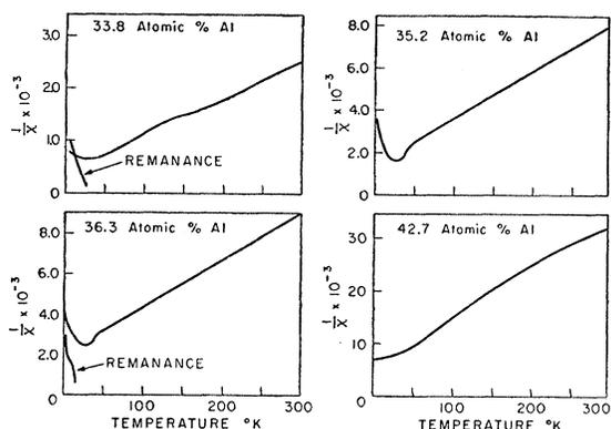
FIG. 5. The inverse susceptibilities of the four cast alloys with higher aluminum contents as functions of temperature. The remanence refers to the magnetization in zero field after magnetizing in an applied field of 12 kilo-oersteds.
