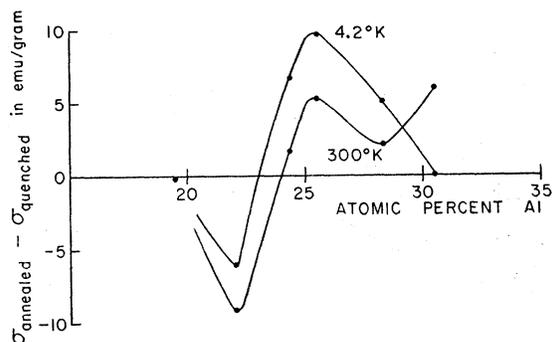
FIG. 4. The differences of spontaneous magnetization between quenched and annealed specimens at 300°K and 4.2°K as a function of aluminum content. Note that the zero value for the 30.5 atomic percent samples result from neither being assumed to have spontaneous magnetization.
