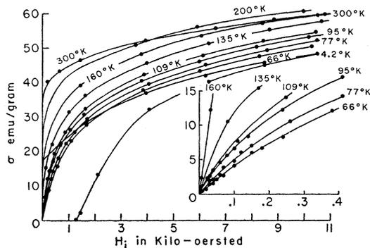
FIG. 8. Magnetization as a function of internal field for several temperatures between 300°K and 4°K for the quenched 30.5 atomic percent specimen. Note the crossing of the 200°K and 300°K isotherms. The 4.2°K isotherm is the same as in Fig. 7.
