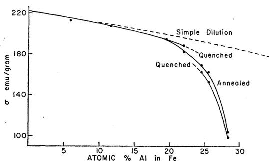
FIG. 3. The spontaneous magnetization at 4.2°K of iron aluminum alloys as a function of composition and heat treatment. Note that the ordinate does not start from zero.
