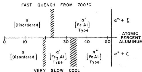
FIG. 1. Schematic diagram of structure resulting from different heat treatments as a function of atomic percent aluminum in iron.
