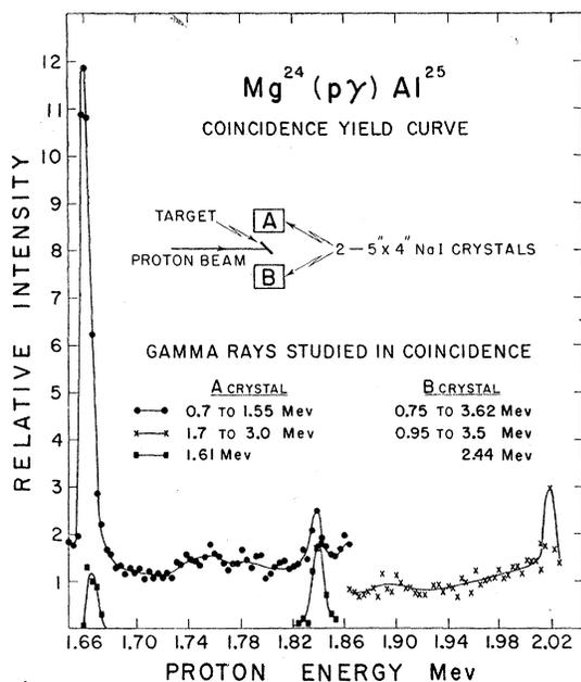
FIG. 1. The yield of gamma rays from the reaction  $Mg^{24}(p,\gamma)Al^{25}$ . The gamma rays were studied in coincidence using two large sodium iodide crystals as shown in the inset. The various ranges of gamma-ray pulse heights studied in coincidence are also shown.
