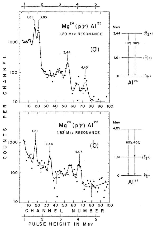
FIG. 3. (a) The gamma-ray pulse spectrum, at  $90^\circ$  to the beam, taken at the 1.20-Mev resonance in the reaction  $Mg^{24}(p,\gamma)Al^{25}$ . The measured<sup>2</sup> branching ratios are shown on the right. (b) The gamma-ray pulse spectrum, at  $90^\circ$  to the beam, taken at the 1.83-Mev resonance in the reaction  $Mg^{24}(p,\gamma)Al^{25}$ . The measured branching ratios are shown on the right.
