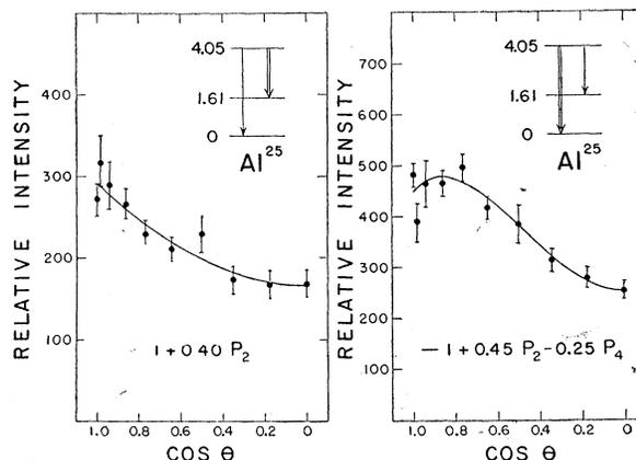
FIG. 4. The angular correlations with respect to the proton beam of the 2.44-Mev gamma rays and the 4.05-Mev gamma rays. The curves are the result of least squares fits to the experimental data. The Legendre polynomial coefficients shown on the figure are also given together with their errors in Table I.
