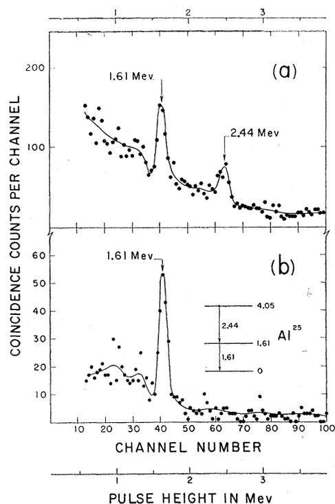
FIG. 2. Coincidence pulse spectra taken at the 1.83-Mev resonance. (a) all gamma-ray pulses in coincidence with gamma-ray pulses in the energy range from 0.75 to 3.62 Mev. (b) All gamma-ray pulses in coincidence with a narrow gate set on the total absorption peak of the 2.44-Mev gamma ray. The inset shows the assumed sequence of the 2.44-Mev and 1.61-Mev gamma rays.
