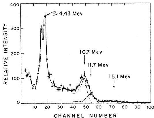
FIG. 11. The pulse distribution of gamma radiation that is coincident with gamma radiation of 4.43-Mev energy from  $He^3$  and  $B^{10}$ . The 10.7-Mev peak is due to the 3.1% cascade branch from the 15.1-Mev state to the 4.43-Mev level. A small yield of 11.7-Mev radiation due to the transition from the 16.1-Mev state to the 4.43-Mev level is also apparent. All of the tail extending out to 15.1 Mev and most of the 4.43-Mev peak is due to chance coincidences.
