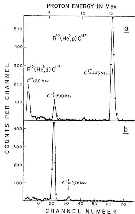
FIG. 5(a). The distribution of pulse heights of particles coincident with all gamma radiation. The groups are labeled by the excitation of the corresponding residual state. The proton energy scale is at the top of the figure. (b) The pulse-height distribution from particles coincident only with radiation above 6.5 Mev in energy.
