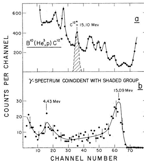
FIG. 7. (a) The particle pulse spectrum showing the voltage gate set on the proton group which corresponds to the formation of the 15.1-Mev state in  $C^{12}$ . (b) The distribution of gamma-ray pulses that are coincident with the particle pulses in the gate shown by the shaded area in (a). Each group is labeled by the corresponding gamma-ray energy.
