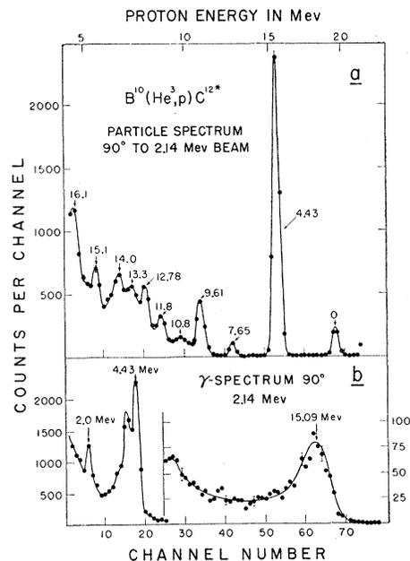
FIG. 2(a). The pulse height spectrum from the CsI particle detector covered by 0.0024 inch of aluminum to stop all alpha particles from  $He^3$  on  $B^{10}$ . Each proton group is labeled by the excitation in Mev of the corresponding state in  $C^{12}$ . The proton energy scale is at the top of the figure. (b) The pulse spectrum from the 5-inch diameter, 4-inch deep NaI gamma-ray detector. Each group is labeled by the energy of the corresponding gamma ray.
