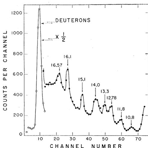
FIG. 3. The pulse-height spectrum from the CsI particle detector with twice the gain but otherwise the same conditions as Fig. 2(a). The very intense group in channel 10 was identified as deuterons from the  $B^{10}(He^3, d)C^{11}$  reaction as discussed in Sec. 3A of the text.
