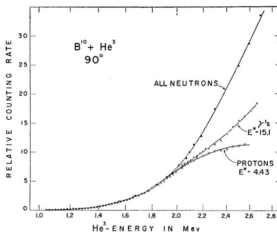
FIG. 4. The excitation curves observed at  $90^\circ$  to beam. The neutron detector was a  $BF_3$  counter surrounded by paraffin<sup>17</sup> for which no absolute efficiency calibration was available. The differential cross sections for the particle groups and gamma radiations are listed in Table I for 2-Mev  $He^3$  bombarding energy.
