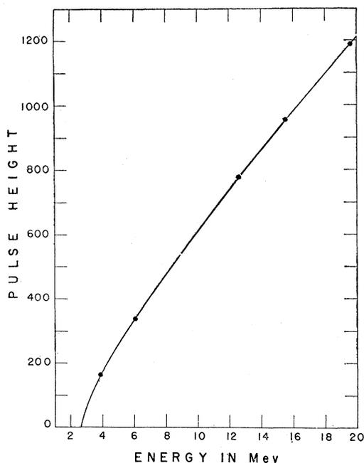
FIG. 1. The proton energy vs pulse-height calibration curve for the CsI particle detector covered by 0.0024 inch of aluminum. The calibration points are discussed in Sec. 2E of the text.
