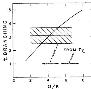
FIG. 14. The values of the intermediate coupling parameter  $a/K$  that are consistent with the measured branching of the 15.1-Mev state. The solid curve is obtained from the calculations of Kurath<sup>15</sup>; the cross-hatched area defines the limits set by the measurements. The range of values of  $a/K$  consistent with the measured width of the ground-state transition<sup>9</sup> is also indicated.
