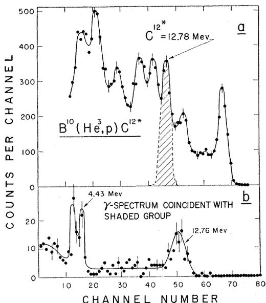
FIG. 8. (a) The particle pulse spectrum showing the voltage gate set on the proton group corresponding to the formation of the 12.78-Mev state in  $C^{12}$ . (b) The distribution of gamma-ray pulses that are coincident with the particle pulses shown by the shaded area in (a). Each group is labeled by the corresponding gamma-ray energy. The 4.43-Mev group is caused by random coincidences and by tail from the corresponding proton group falling in the gate.
