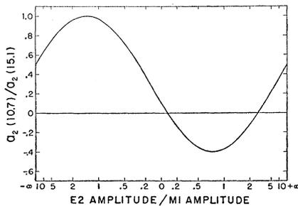
FIG. 15. The computed ratio of the  $a_2$  coefficients of the 10.7-Mev radiation to that of the 15.1-Mev radiation as a function of the multipole mixture in the 10.7-Mev gamma radiation. The angular distributions are each assumed normalized to the form  $1+a_2P_2(\cos\theta)$ .
