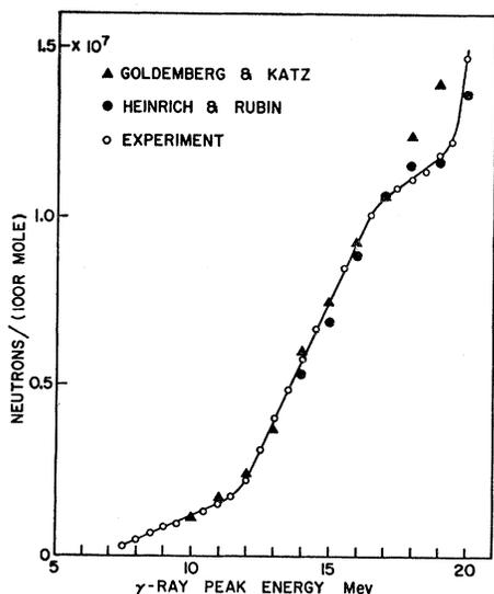
Fig. 3.  $(\gamma, n)$  yield from  $\text{Li}^7$  as a function of  $\gamma$ -ray peak energy.
