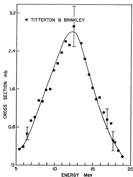
FIG. 5.  $(\gamma, n)$  cross section for  $\text{Li}^6$  as a function of  $\gamma$ -ray energy.
