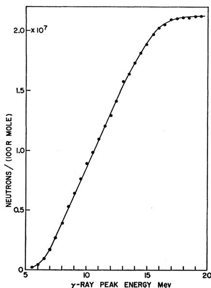
Fig. 4.  $(\gamma, n)$  yield from  $\text{Li}^6$  as a function of  $\gamma$ -ray peak energy.
