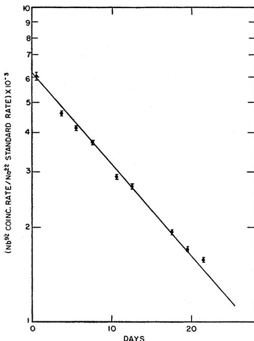
FIG. 4. Positron decay observed by 511–511 kev gamma-ray coincidences in two NaI crystals. The indicated decay curve has the 10.15-day Nb<sup>92</sup> half-life.
