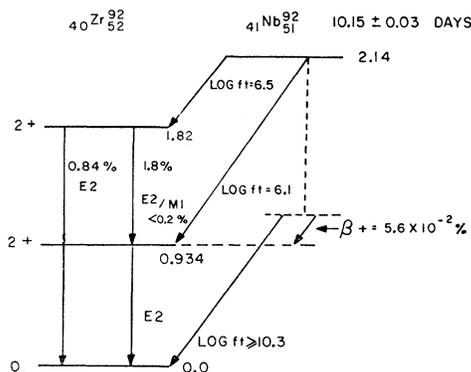
FIG. 1. Decay scheme of Nb<sup>92</sup>.
