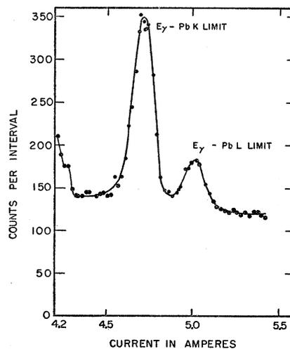
FIG. 3. Energy spectrum of the conversion electrons ejected from a 0.5-mil Pb radiator by the gamma rays in  $\text{Nb}^{92}$  decay, observed by a thin lens spectrometer.
