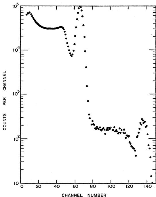
FIG. 2. NaI pulse-height spectrum of the gamma rays in the decay of  $\text{Nb}^{92}$ .
