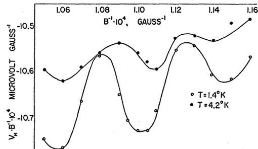
FIG. 13. Temperature variation of the oscillatory component of the Hall effect for crystal  $ac-1$ ,  $J||a$ -axis,  $B||c$ -axis.
