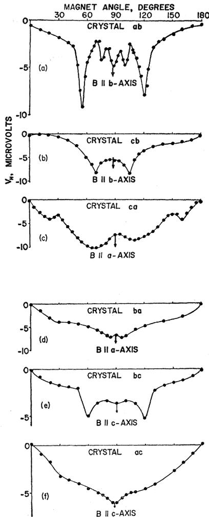
FIG. 6. Hall voltage rotation curves for gallium single crystals at 4.2°K; (a)  $J \parallel a$ -axis,  $B$  in  $bc$  plane, (b)  $J \parallel c$ -axis,  $B$  in  $ab$  plane, (c)  $J \parallel c$ -axis,  $B$  in  $ab$  plane, (d)  $J \parallel b$ -axis,  $B$  in  $ac$  plane, (e)  $J \parallel b$ -axis,  $B$  in  $ac$  plane, and (f)  $J \parallel a$ -axis,  $B$  in  $bc$  plane. All of the rotation curves are for a field of 9.6 kgauss.
