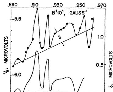
FIG. 12. Oscillations in Hall voltage for crystal  $ba$ ,  $J||b$ -axis,  $B||a$ -axis,  $T=1.4^\circ\text{K}$ .
