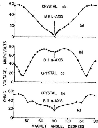
FIG. 7. Magnetoresistance rotation curves for gallium single crystals at 4.2°K; (a)  $J \parallel a$ -axis,  $B$  in  $bc$  plane, (b)  $J \parallel c$ -axis,  $B$  in  $ab$  plane, (c)  $J \parallel b$ -axis,  $B$  in  $ac$  plane. All of the rotation curves are for a field of 9.6 kgauss.
