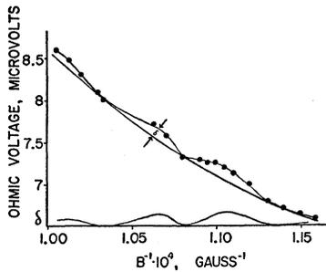
FIG. 11. Oscillations in magnetoresistance for crystal  $ac$ ,  $J||a$ -axis,  $B||c$ -axis,  $T=1.4^\circ\text{K}$ .
