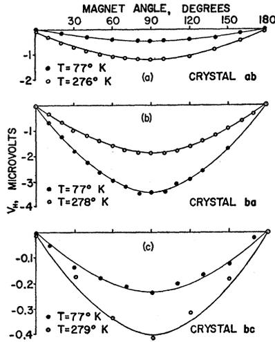
FIG. 2. Hall voltage rotation curves for gallium single crystals at 77°K and 290°K; (a)  $J \parallel a$ -axis,  $B$  in  $bc$  plane, (b)  $J \parallel b$ -axis,  $B$  in  $ac$  plane, (c)  $J \parallel b$ -axis,  $B$  in  $ac$  plane. All of the rotation curves are for a field of 9.6 kgauss.
