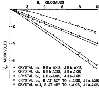
FIG. 4. Hall voltage field dependence for gallium single crystals at 4.2°K. Note that the dependence is linear above 3 kgauss but that below this field a nonlinear dependence seems indicated.
