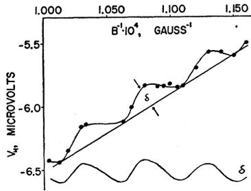
FIG. 10. Oscillations in Hall voltage for crystal  $ac$ ,  $J||a$ -axis,  $B||c$ -axis,  $T=1.4^\circ\text{K}$ .
