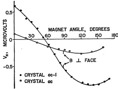
FIG. 3. Shift in the maximum of the Hall rotation curve for crystals *ac* and *ac-1* at 77°K. Here  $J \parallel a$ -axis and  $B (=9.6 \text{ kgauss})$  is in the *bc* plane. (Crystal *ac-1* has a larger misorientation of crystallographic axes from specimen axes than crystal *ac* with a correspondingly larger shift, see Text.)
