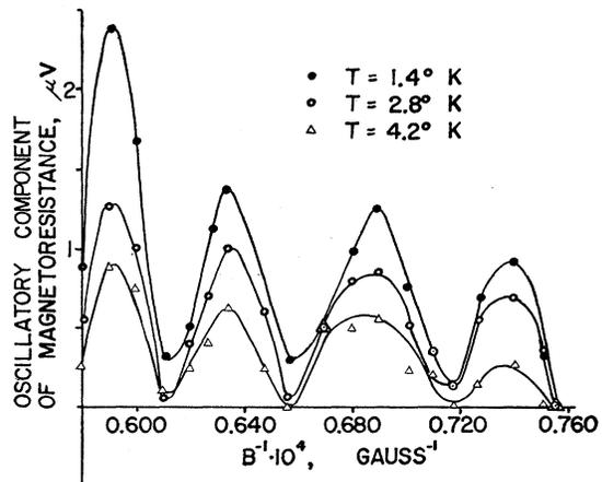
FIG. 14. Temperature variation of the oscillatory component of the magnetoresistance for crystal  $ac$ ,  $J||a$ -axis,  $B||c$ -axis.
