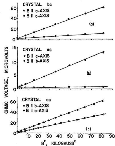
FIG. 5. Field dependence of magnetoresistance for gallium single crystals at 4.2°K; (a)  $J \parallel b$ -axis, (b)  $J \parallel a$ -axis, (c)  $J \parallel c$ -axis.
