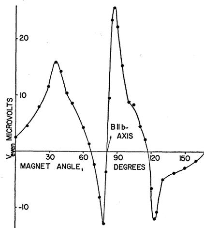
FIG. 9. Rotation curve of quadratic transverse effect for crystal  $ab$ -1 at 1.4°K,  $J \parallel a$ -axis and  $B (= 11.2 \text{ kgauss})$  is in the  $bc$  plane. The ordinate is the sum of the pure quadratic voltage in  $B$  and the even voltage due to a resistive component associated with a longitudinal misalignment of the Hall probes. For this crystal, the crystallographic axes and specimen axes are misaligned by about  $10^\circ$ .
