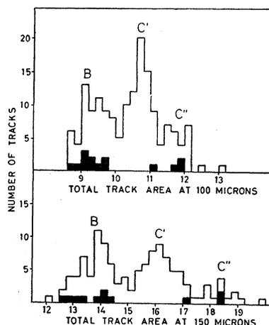
FIG. 3. Histogram showing the total track area, in arbitrary units, of the fragments in group *C* of Fig. 2. The measurements are made by means of a "Xenon-Hochdruckbrenner."
