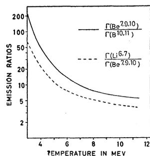
FIG. 24. The theoretical ratios  $(\text{Li}^6 + \text{Li}^7)/(\text{Be}^7 + \text{Be}^9 + \text{Be}^{10})$  and  $(\text{Li}^6,7)/(\text{Be}^7 + \text{Be}^9 + \text{Be}^{10})$  as functions of the temperature  $T$ , calculated from nuclear evaporation theory. Only fragments of range  $> 100 \mu$  are considered.
