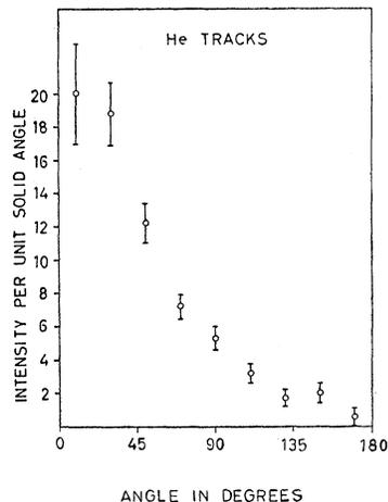
FIG. 8. Angular distribution of fast helium nuclei of kinetic energy  $>45$  Mev.
