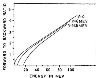
FIG. 21. Theoretical "forward to backward" ratios for  $\text{Li}^8$  fragments calculated from (3a,b) with  $T=11.5$  Mev,  $v=0.016c$ , and three different values of  $V$ .
