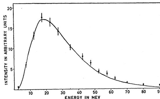
FIG. 5. Observed energy spectrum of  $Li^8$  "hammer" tracks. The curve is calculated from the formulas (2a,b) with  $T=11.5$  Mev,  $V=6$  Mev and  $v=0.016c$ .
