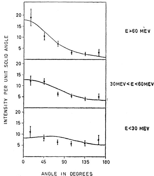
FIG. 9. Angular distribution of  $(\text{Li}^6, \text{Li}^7)$  and  $\text{Li}^8$  fragments, grouped together, for three different intervals of kinetic energy. The curves are calculated from the formula (5) with  $T=11.5$  Mev,  $V=6$  Mev, and  $v=0.016c$ .
