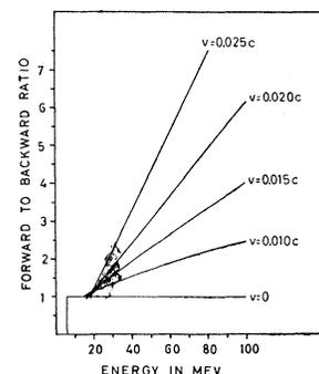
FIG. 23. Theoretical "forward to backward" ratios for  $\text{Li}^8$  fragments calculated from formula (3a,b) with  $T=11.5$  Mev,  $V=6$  Mev, and different values of  $v$ .
