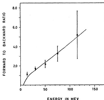
FIG. 11. The observed "forward to backward" ratio for  $(\text{Li}^6, \text{Li}^7)$  and  $\text{Li}^8$  fragments grouped together as a function of energy. The curve shows the theoretical  $F/B$  ratios for  $\text{Li}^8$  calculated from (3a,b) with  $T=11.5$  Mev,  $V=6$  Mev, and  $v=0.016c$ .
