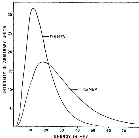
FIG. 18. Theoretical energy spectra of  $\text{Li}^8$  fragments calculated from formula (2a,b) with  $V=6$  Mev,  $v=0.016c$ , and  $T=6$  Mev and 11.5 Mev, respectively.
