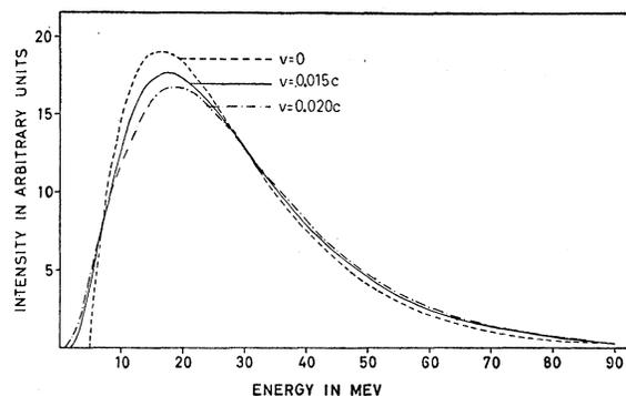
FIG. 22. Theoretical energy spectra of  $\text{Li}^8$  fragments calculated from formula (2a,b) with  $T=11.5$  Mev,  $V=6$  Mev, and three different values of  $v$ .
