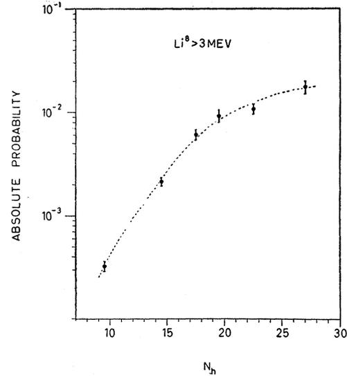
FIG. 16. The absolute probability of emission of  $\text{Li}^8$  fragments of energy  $> 3$  Mev as a function of  $N_h$ .
