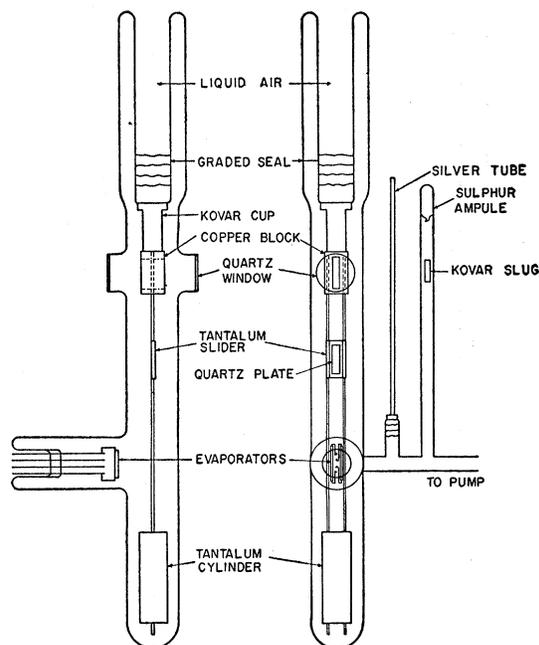
FIG. 1. Construction of optical absorption tube.
