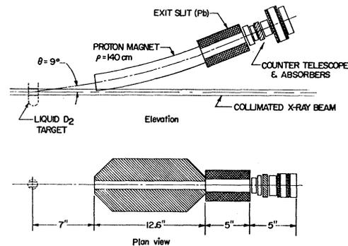
FIG. 1. Elevation view of the target, magnet, and counter telescope arrangement for the  $11^\circ$  c.m. measurement.
