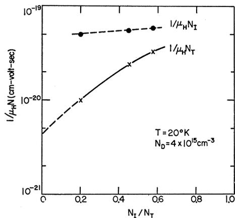
FIG. 9. Dependence of  $1/\mu_H N_I$  and  $1/\mu_H N_T$  upon the fraction of ionized to total impurities.
