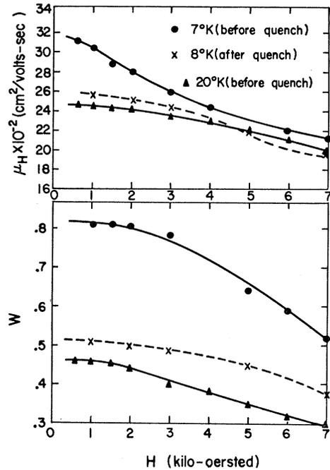
FIG. 5. The magnetic field dependence of the function *W* and the Hall mobility, showing the influence of additional ionized impurities at low temperature.
