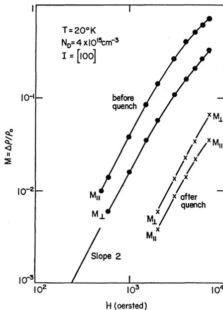
FIG. 7. Magnetic field dependence of magnetoresistance for uncompensated and heavily compensated  $n$ -type Ge.
