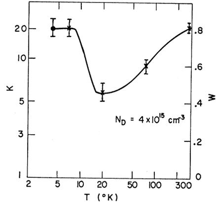
FIG. 4. Temperature dependence of the effective anisotropy parameter *K*.
