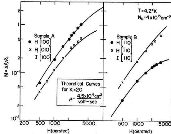
FIG. 10. The magnetic field dependence of magnetoresistance of optically excited electrons, compared with high-field theory of Abeles and Meiboom.
