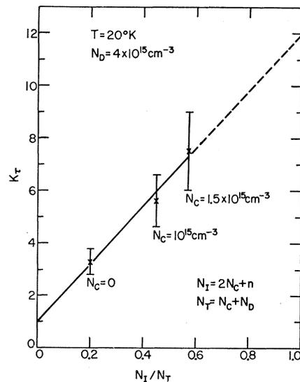
FIG. 8. Scattering anisotropy parameter  $K_\tau$  as a function of fraction of ionized to total impurities for increasing concentration of compensating impurities.
