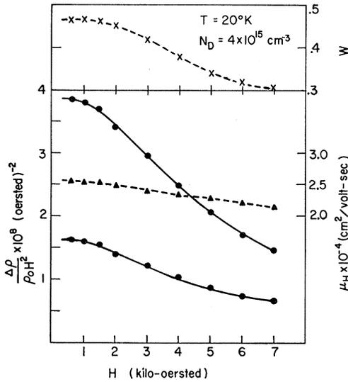
FIG. 3. The magnetic field dependence of magnetoresistance, Hall mobility, and function *W* for an uncompensated sample.
