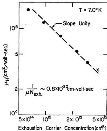
FIG. 6. Hall mobility of electrons at low temperature as a function of exhaustion carrier concentration. Solid points from unpublished data of H. Fritzche.
