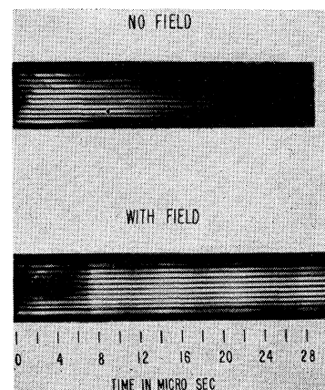
FIG. 8. Shock collision in a 20 cm H-tube with 200 microns deuterium and H_{\text{max}} = 60\,000 gauss. The reduced luminosity after collision is due to lower impurity concentrations from wall vaporization with a confining field. Radiation from silicon and oxygen produces most of the light in the no (axial) field case and in the bursts of light from the ringing of the field coil.
