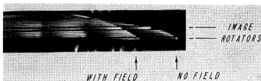
FIG. 6. Smear camera photographs with and without confining field (double exposure) showing radial compression and the stability of the confined plasma. The time and distance scale are the same as in Fig. 5. The velocity falls off rapidly as the field decreases in magnitude. The ambient pressure was 400 microns deuterium with a maximum field of 15 000 gauss.
