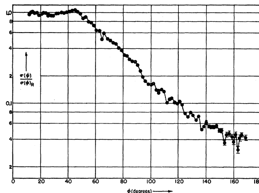
FIG. 4. Elastic scattering of 18.70-Mev alpha particles by Ag. The Rutherford cross section is given by \sigma(\Phi)_R = 35.1 \text{ csc}^4(\Phi/2) \text{ mb/sterad} .
