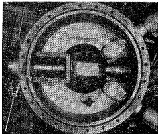
FIG. 4. Multiple exposure photograph of the apparatus with vacuum-tight lid removed. A frosted lamp placed at the source position reveals the beam direction (using smoke with foil removed) and the region of impact on the Deltamax foil (using translucent paper).
