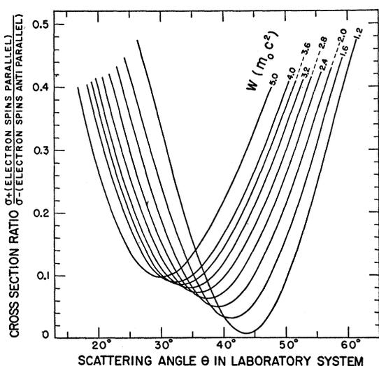
FIG. 1. Theoretical scattering cross-section ratios for longitudinally polarized electrons incident upon target electrons which are polarized parallel or anti-parallel to the direction of incidence.  $W$  is the total energy of the incident electrons in units of  $m_0 c^2$ .
