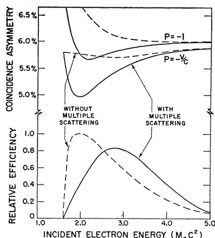
FIG. 2. Predicted effects for monoenergetic electrons in the experimental arrangement used. In the upper part coincidence asymmetries are plotted for full polarization ( $P = -1$ ) and a  $-v/c$  polarization ( $P = -v/c$ ). The broken lines were computed without taking multiple scattering into account. The solid curves are the result of the approximate graphical analysis discussed in the text.
