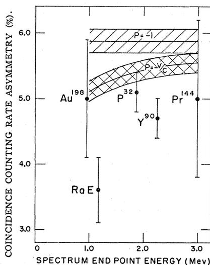
FIG. 6. Plot of the polarization results as a function of beta-spectrum end-point energy.
