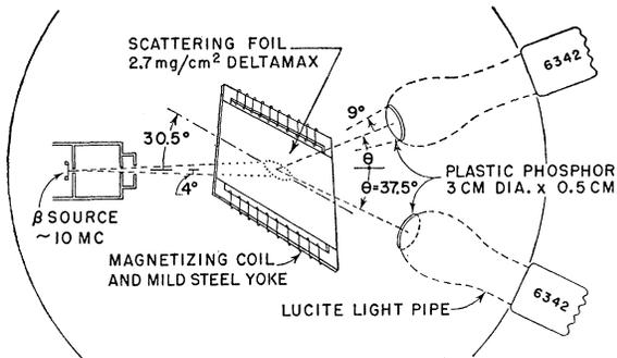
FIG. 3. Schematic diagram of Møller scattering apparatus.
