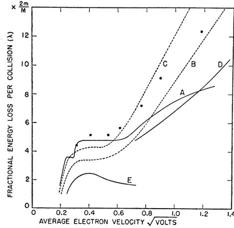
FIG. 6. The fractional energy loss of an electron per collision with a hydrogen molecule as a function of the electron velocity. Curve A, present microwave measurements; curve B, Crompton and Sutton's shower experiments for a Maxwellian distribution of electron velocities; curve C, assumed Druyvesteyn distribution; curve D, calculated with no assumptions; curve E, theoretical (Gerjuoy and Stein); the solid dots are from measurements of Townsend and Bailey.
