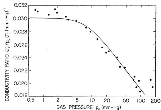
Fig. 1. Conductivity ratio as a function of the gas pressure. ● measurements; the solid line is obtained from theory for  $P_m = 28(v/v_0)^{0.6}$  (cm-mm Hg)<sup>-1</sup>.
