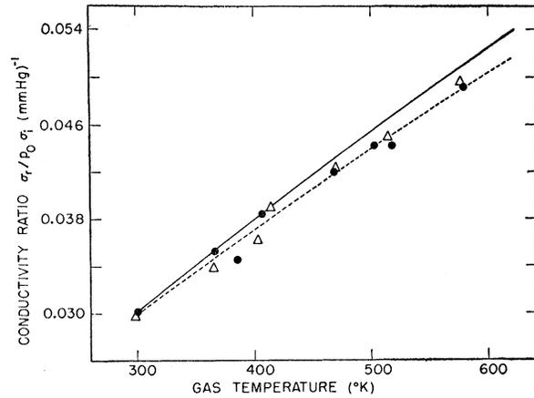
Fig. 2. Conductivity ratio as a function of the gas temperature. ● measurements in hydrogen; △ measurements in deuterium; the solid line is obtained from theory for  $P_m = 28(v/v_0)^{0.6}$ ; the dashed line is obtained from theory for  $P_m = 29(v/v_0)^{0.5}$  (cm-mm Hg)<sup>-1</sup>.
