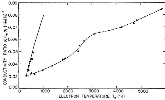
FIG. 3. Comparison between the conductivity ratio obtained by thermal agitation of the electrons ( $\bullet$ ) with that obtained by microwave agitation ( $-\triangle-\triangle-$ ). The solid line is obtained from theory for  $P_m = 28(v/v_0)^{0.6}$  ( $\text{cm-mm Hg}$ ) $^{-1}$ .
