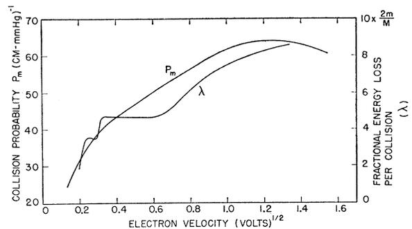
FIG. 4. Collision probability for momentum transfer  $P_m$ , and the fractional energy loss  $\lambda$  per collision, as a function of the electron velocity.
