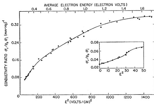
FIG. 5. Measured conductivity ratio ( $-\bullet-$ ) as a function of the root-mean-square value of the microwave electric field used in heating the electrons. The computed average electron energy is also given.
