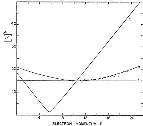
FIG. 4. The square roots of the "shape factors" are plotted vs the momentum. Momentum is in relativistic units (units of  $mc$ ). Curve I represents the shape factor for an allowed spectrum; Curve II, for a first-forbidden spectrum with  $\Delta J=0$ ; Curve III, for a first-forbidden spectrum with  $\Delta J=2$ . The scales are adjusted to give an intersection point at  $p=10.5$ . The circles represent the empirical correction factors.
