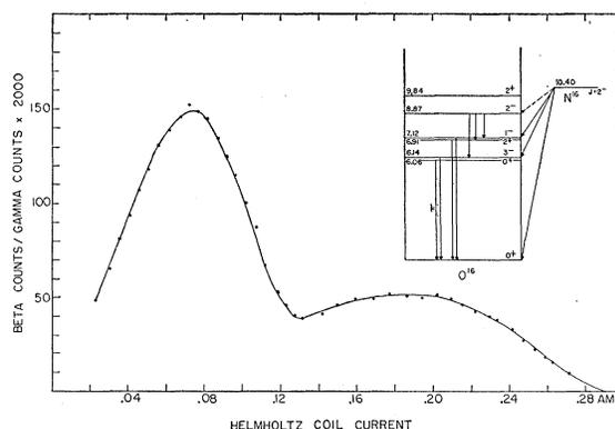
FIG. 1. Spectrum of beta rays from  $N^{16}$  decay. The probable error is approximately represented by twice the size of the points. The insert indicates the pertinent known energy levels of  $O^{16}$ .
