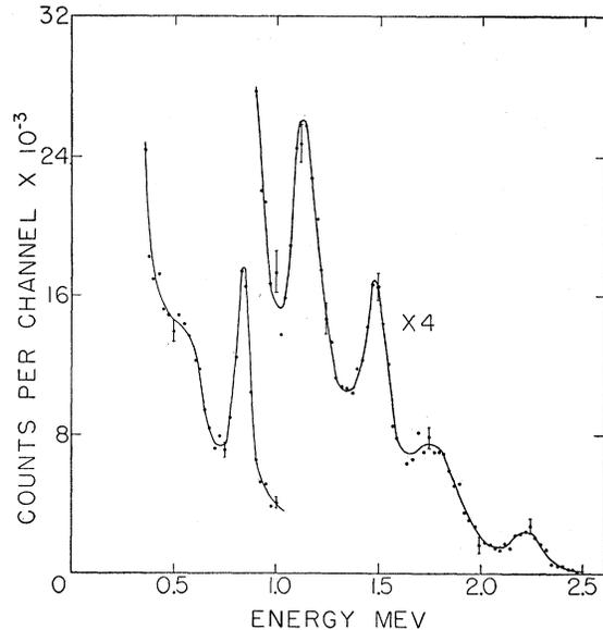
FIG. 2. Upper energy portion of  $Mn^{55}$  gamma spectrum.
