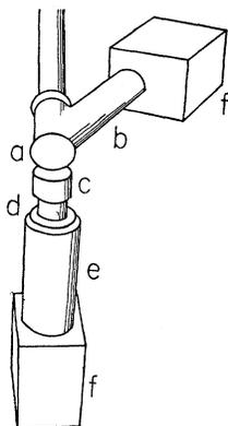
FIG. 1. Scattering geometry for gamma-ray experiments, showing: *a*, target; *b*, proton monitor; *c*, scatterer; *d*, scintillation crystal; *e*, photomultiplier tube; *f*, preamplifiers.
