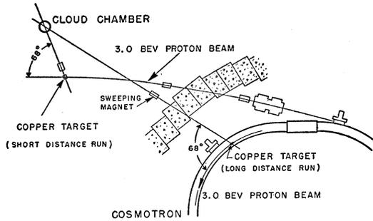
FIG. 1. Experimental arrangements for lifetime study.
