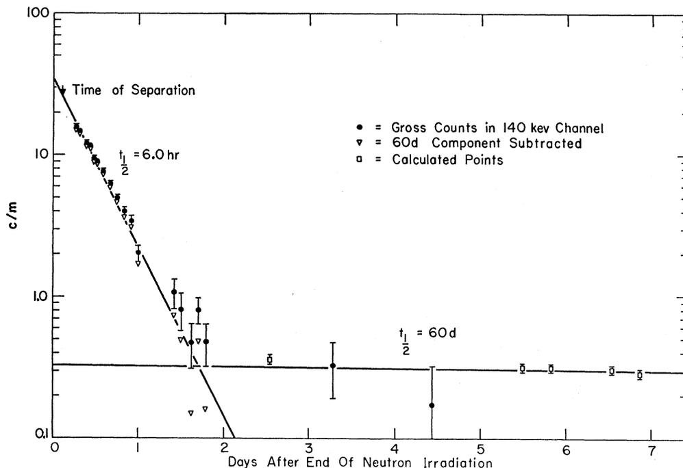
FIG. 1. Sample *A*. Decay curve of technetium fraction after neutron irradiation. After the decay of 6-hr  $Tc^{99m}$ , several calculated points at 140 kev were obtained by multiplying the 201-kev counting rate of the sample by the ratio of the 140-kev/201-kev counting rates of a strong  $Tc^{99}$  source.
