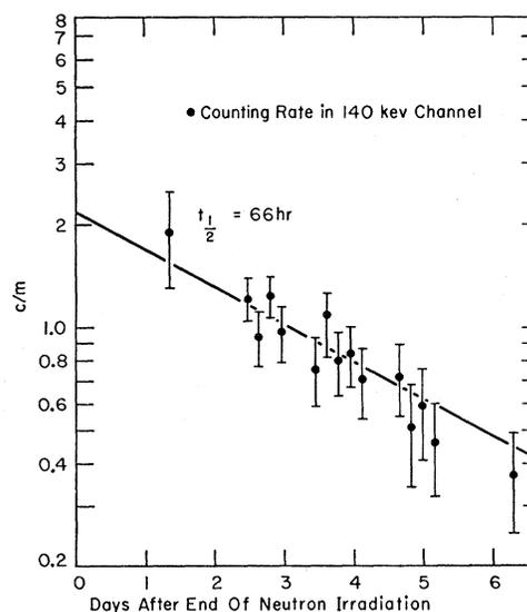
FIG. 2. Sample A. Decay curve of molybdenum fraction after neutron irradiation.
