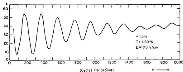
FIG. 2. A typical experimental curve of current *I* reaching the collector vs the frequency  $\nu$  of the ac field between each shutter. In practice such a curve is traced out on a recording meter connected to the electrometer output while the oscillator frequency is slowly swept by a clock motor.
