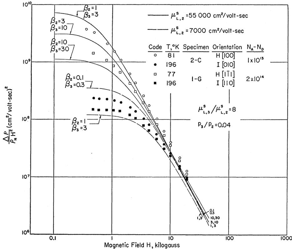
FIG. 5. Comparison of theoretical transverse magnetoresistance coefficients (solid lines and broken lines) with experimental data on germanium (isolated points) at liquid nitrogen and dry ice temperatures.
