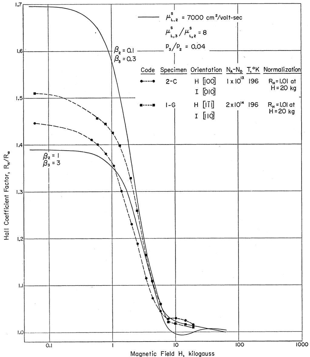
FIG. 4. Comparison of theoretical Hall coefficient factor (solid lines) with experimental data on germanium (dashed lines) for a temperature of 196°K.
