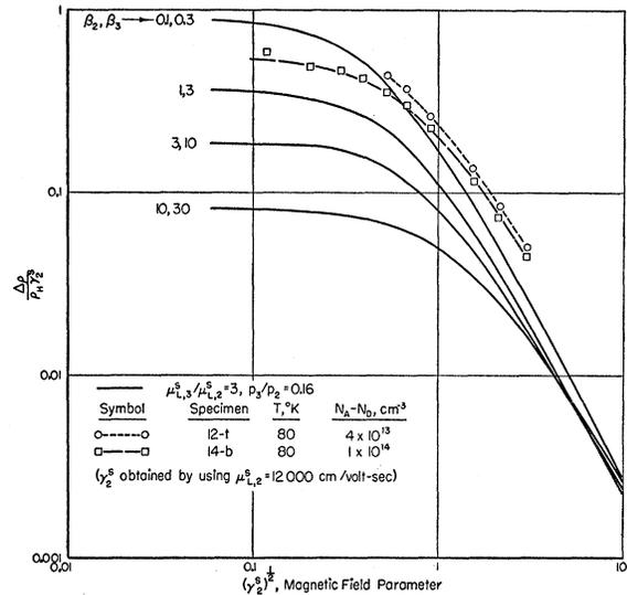
FIG. 7. Comparison of theoretical transverse magnetoresistance coefficients (solid lines) with experimental data on silicon (dashed and broken lines) at 80°K.
