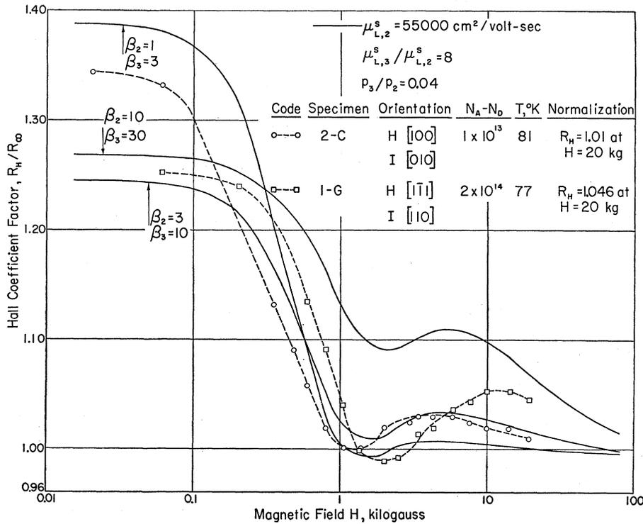
FIG. 3. Comparison of theoretical Hall coefficient factor (solid lines) with experimental data on germanium (dashed lines) for liquid nitrogen temperatures.
