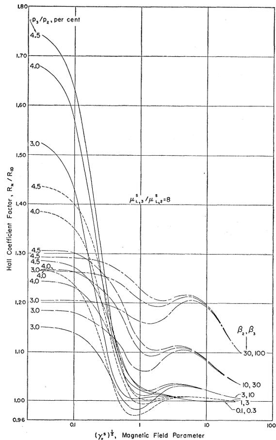
FIG. 2. Hall coefficient factor for degenerate valence bands representative of germanium. Parameters are density ratios of light and heavy holes, and impurity scattering factors.
