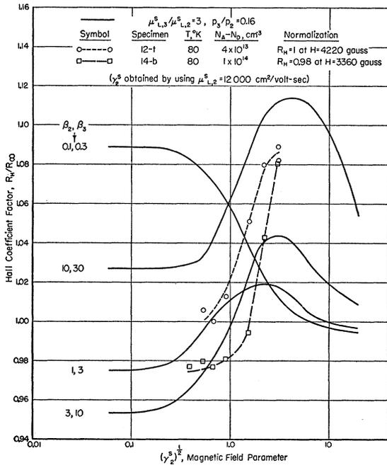
FIG. 6. Comparison of theoretical Hall coefficient factor (solid lines) with experimental data on silicon (dashed and broken lines) for a temperature of 80°K.
