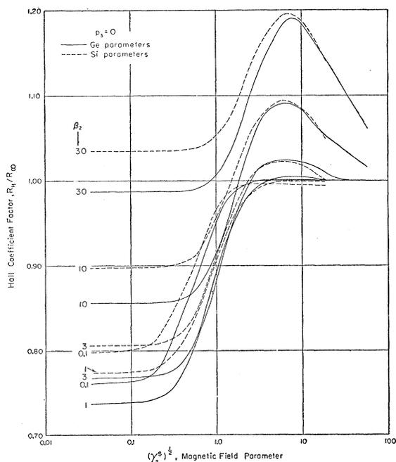
FIG. 1. Hall coefficient factor for a single warped band. The solid lines are for parameters representative of the heavy-mass band in germanium as determined from cyclotron resonance. The dashed lines are applied to silicon. The parameter  $\beta_2$  measures the degree of impurity scattering.
