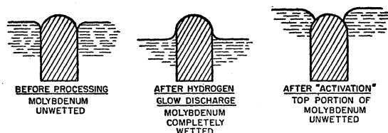
Fig. 2. Shape of mercury meniscus.
