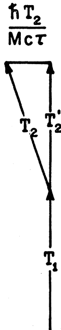
FIG. 2. The emission of a light signal confined to a time interval \tau produces a recoil in the motion of the clock. As a result, the clock will proceed along the arrow marked T_2 . The true distance between the tip of this arrow and the original position of the clock, at the bottom of the figure, differs from the indication T_1+T_2 of the clock.
