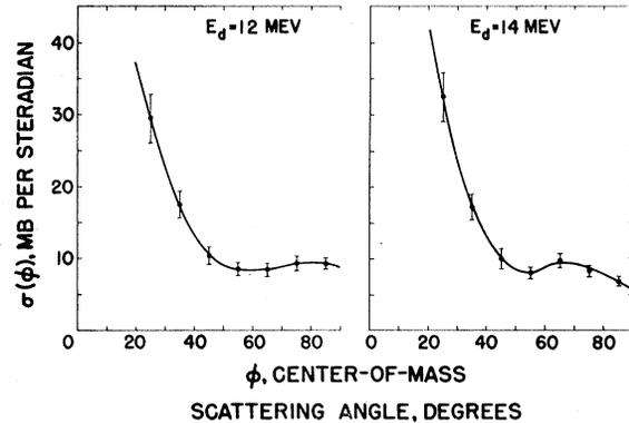
FIG. 6. c.m. angular distribution, integrated over energy, for the  $He^3$  particles from 12- and 14-Mev deuterons on tritium.
