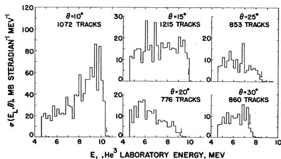
FIG. 3. Energy spectrum of continuum of doubly charged particles from 14-Mev deuterons on tritium for various laboratory angles.
