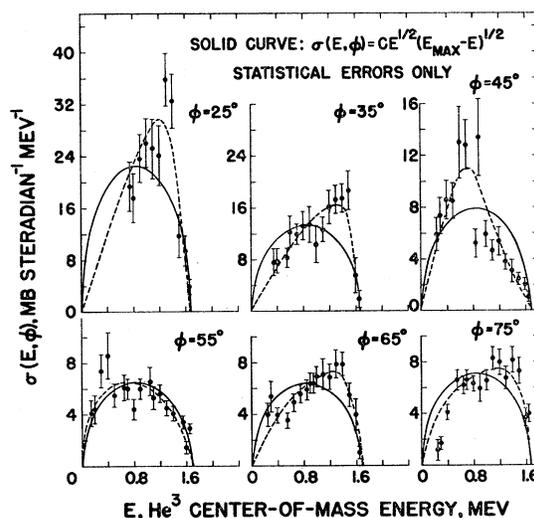
FIG. 4. c.m. energy distribution, for various c.m. angles, for the  $\text{He}^3$  particles from the  $T(d,2n)\text{He}^3$  reaction for 12-Mev deuterons.
