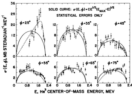
FIG. 5. c.m. energy distribution, for various c.m. angles, for the  $He^3$  particles from the  $T(d,2n)He^3$  reaction for 14-Mev deuterons.
