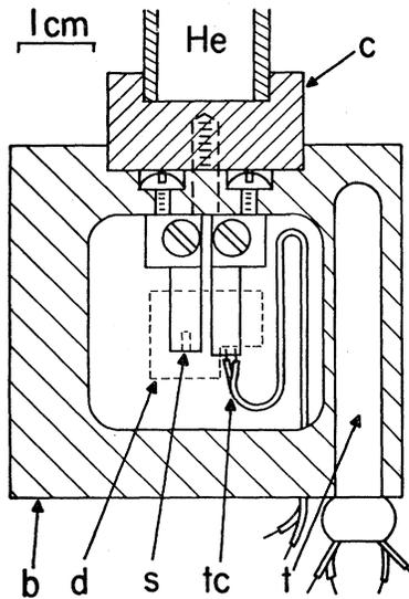
FIG. 2. Vertical section of specimen block assembly.  $c$  = tail of cryostat,  $b$  = OFHC copper block,  $d$  = cross section of deuteron beam,  $s$  = region on specimen crystal studied by x-rays,  $tc$  = dummy foil thermocouple,  $t$  = platinum resistance thermometer. The block has front and back faceplates as thermal radiation shielding for the specimen; the deuteron and x-ray ports subtend only about  $\pi/3$  steradian.
