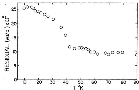
Fig. 4. Thermal recovery of irradiation-induced lattice expansion.
