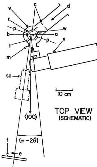
distribution  $\Delta\lambda \approx 0$  and for large  $\theta$  the shift in angle,  $\Delta\theta$ , becomes a sensitive measure of lattice expansion. In the present experiment  $\text{Co } K\alpha_1$  radiation and a  $\{400\}$  reflection were used. At 10°K,  $\theta = 83^\circ 10'$  and  $\tan\theta = 8.345$ ; this choice of reflecting planes and characteristic radiation affords the highest sensitivity readily available for copper at low temperature.
