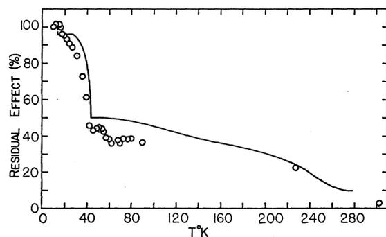
FIG. 7. Thermal recovery of deuteron damage in copper.  $\circ$  The present lattice expansion measurements; — electrical resistivity (Cooper *et al.*,<sup>3</sup> Run II; --- indicates the effect of an initial one-minute temperature pulse to near 30°K).
