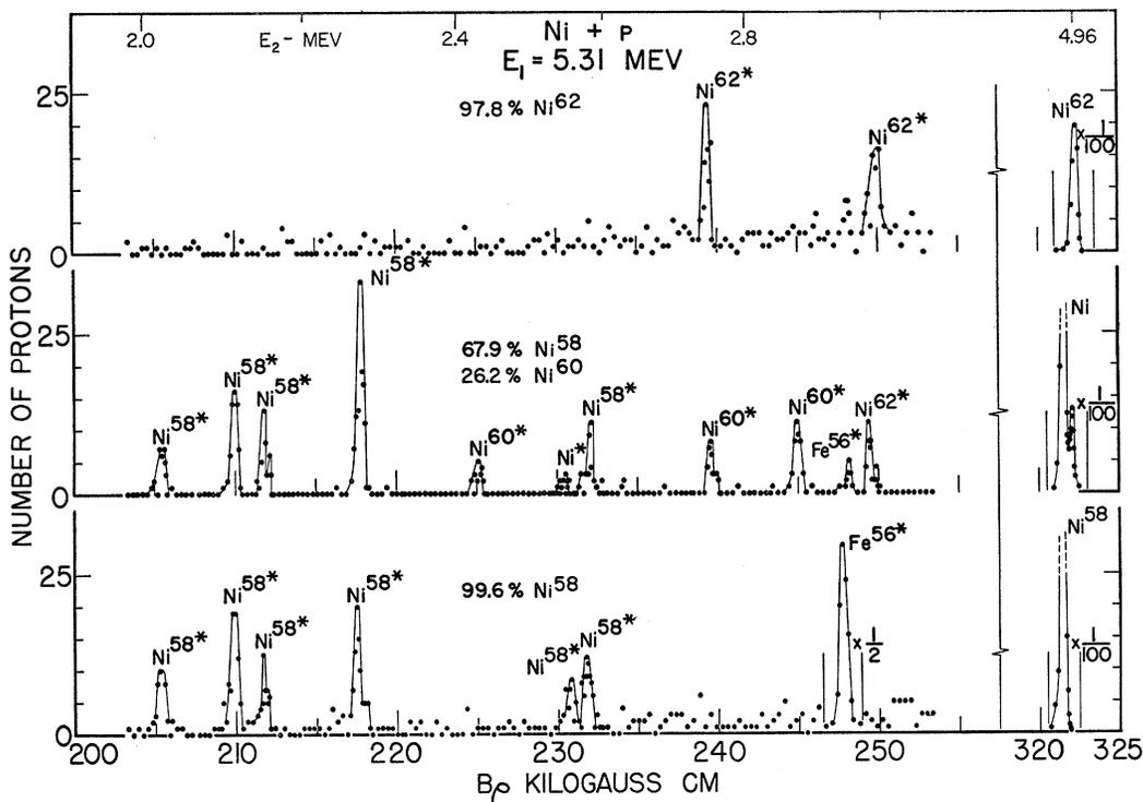
FIG. 3. Partial spectra of protons scattered from targets of nickel oxide enriched to 97.8% in  $\text{Ni}^{62}$  and nickel oxide enriched to 99.6% in  $\text{Ni}^{58}$  and evaporated on carbon foils, and a natural nickel foil. Protons from excited states above 2.0 Mev in nickel are shown. The scale at the top gives the energy  $E_2$  of the scattered protons.
