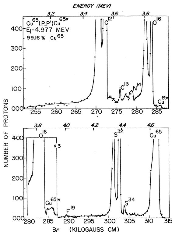
FIG. 1. Partial spectrum of protons scattered from an evaporated target enriched to 99.16% in  $\text{Cu}^{65}$  and showing the proton group from the state at 0.768 Mev of excitation in  $\text{Cu}^{65}$ . The scale at the top of each figure gives the energy  $E_2$  of the scattered protons.
