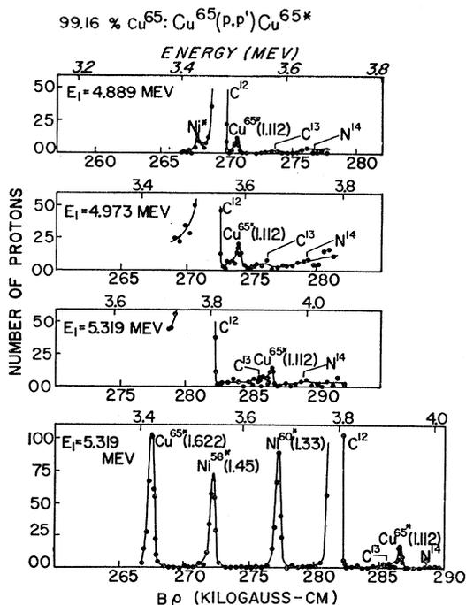
FIG. 2. Partial spectra of protons scattered from an evaporated target enriched to 99.16% in  $\text{Cu}^{65}$ . The upper three spectra are those used to identify the state at 1.112 Mev of excitation. The lower spectrum shows a proton group from the state at 1.622 Mev.
