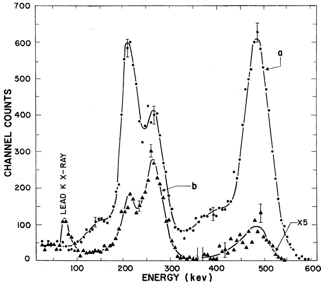
FIG. 6. Gated scintillation spectrum of  $As^{77m}$  decay (background has been subtracted). Curve *a*—Source in  $\frac{1}{4}$ -in. Lucite beta absorber. Curve *b*—Source in 0.24-cm lead absorber to reduce the addition peak of the 210- plus 265-kev gamma rays.
