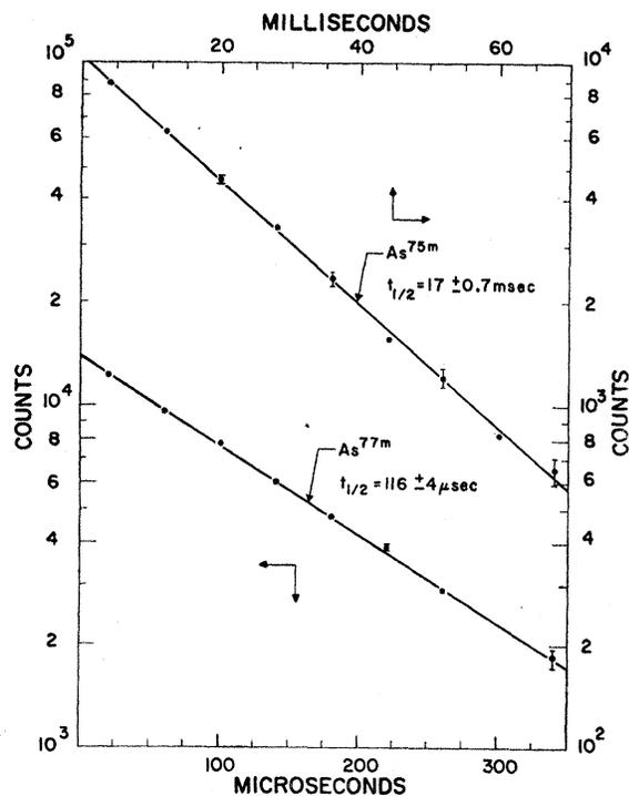
FIG. 4. Gamma-ray decay curves of  $As^{75m}$  and  $As^{77m}$  (accidental coincidence background has been subtracted). The  $As^{75m}$  curve is to be read on the right and upper scales; the  $As^{77m}$  curve is to be read on the left and lower scales.
