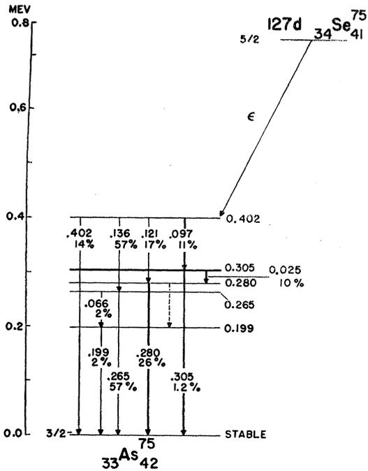
FIG. 2. Decay scheme of  $\text{Se}^{75}$ . Level and transition energies are given in Mev. Transitions involving the isomeric state at 0.305 Mev are shown with heavy lines.
