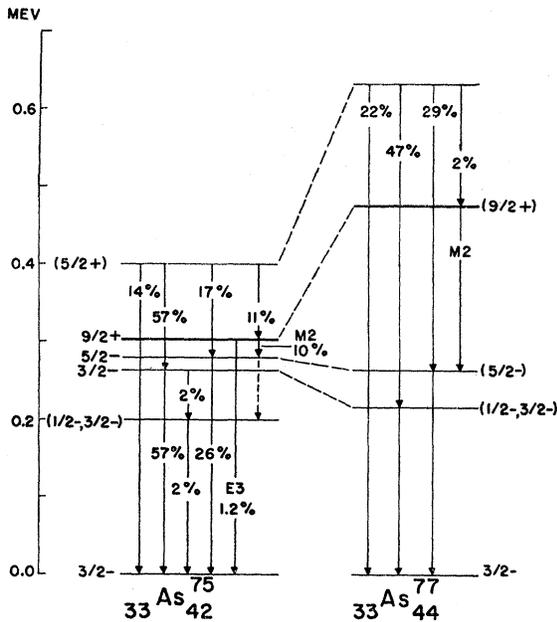
FIG. 8. Comparison of  $As^{76}$  and  $As^{77}$  level schemes. Transition intensities are given in percentage of the 402- and 632-keV level decays, respectively.
