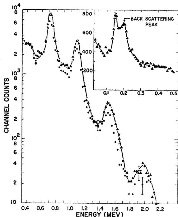
FIG. 5. Gated scintillation spectrum of gamma rays in the  $\text{Ge}^{77}$  decay which feed  $\text{As}^{77m}$  (accidental coincidence background has been subtracted).  $\blacktriangle$  source surrounded by  $\frac{1}{2}$ -in. Lucite beta absorber.  $\bullet$  source surrounded by tin absorber to reduce 153-keV peak. Insert, low-energy region taken with  $\text{Ge}^{77}$  source in Lucite absorber.
