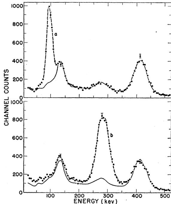
FIG. 3. Pulse-height spectrum of a  $\text{Se}^{75}$  source at the center of a well-type  $\text{NaI}(\text{Tl})$  crystal. Solid curves, ungated spectra normalized to give accidental background under gated spectra. Curve *a*—15-msec delayed coincidence spectrum superimposed on accidental background displaying gamma rays feeding the isomeric state. Curve *b*—Gated spectrum displaying gamma rays due to isomeric decay.
