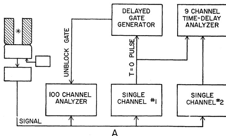
FIG. 1. Block diagram of delayed coincidence circuits. Diagram A—Arrangement for measuring isomeric half-life and the scintillation pulse-height spectrum of the gamma rays leaving the isomeric state. Diagram B—Arrangement for measuring the pulse-height spectrum of the gamma rays feeding the isomeric state.
