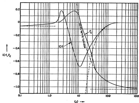
FIG. 1. The functions  $10f(\omega)$  and  $\Gamma_C(\omega)$  which determine the dispersive and absorptive parts of the Delbrück forward scattering amplitude for Pb. The semiempirical description of pair production by Davies, Bethe, and Maximon is indicated. The asymptotic forms are drawn as dashed lines.
