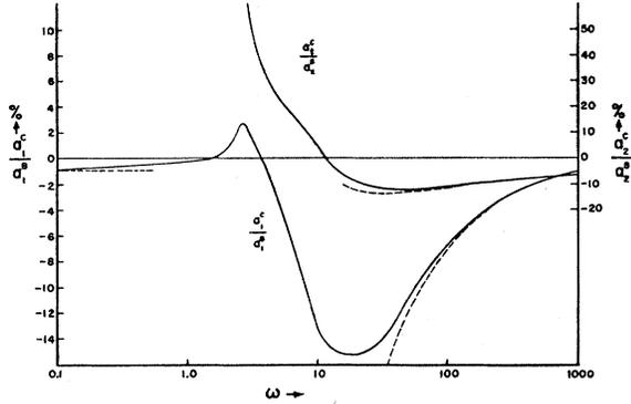
FIG. 2. Coulomb corrections for Pb to the dispersive part ( $a_1^B$ ) and absorptive part ( $a_2^B$ ) of the forward scattering amplitude in Born approximation. Note that different scales apply in the two cases. The dashed lines are the asymptotic values.
