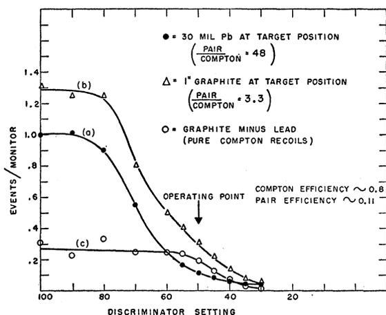
FIG. 3. Pulse-height spectra from (a) lead in target position (pure pairs), (b) carbon in target position (pairs +  $\sim 25\%$  Comptons), and (c) the difference between (b) and (a). Curve (c) shows no pair characteristics and is clearly the response of our apparatus to pure Compton recoils.
