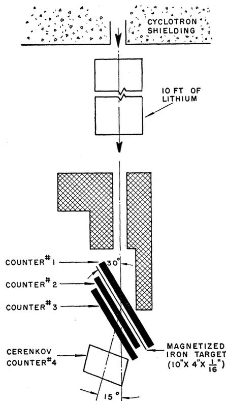
FIG. 1. Apparatus for counting Compton recoils from high-energy photons. Reversal of magnetization in the iron plate allows a measurement of the degree of circular polarization of the  $\pi^0$ -decay photons. Pairs are rejected by using as the "event" counts (12343') with pulses 3' being all those pulses from 3 larger than a given discriminator setting.
