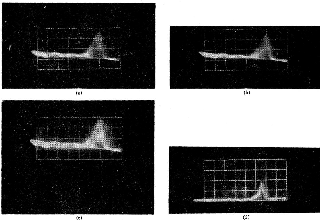
FIG. 2. Pulse-height spectra in counter 3. (a) Pulses from a lead foil at the target position, which give  $(\bar{1}234)$  coincidence; (b) pulses primarily from single electrons incident, which give  $(234)$  coincidence; (c) pairs plus singles  $(234)$ , with lead foil in target position; (d) pulse spectrum of  $c$ , but with anticoincidence  $(234\bar{3}')$  showing the pulse-height spectrum of the pulses which we count as Comptons.
