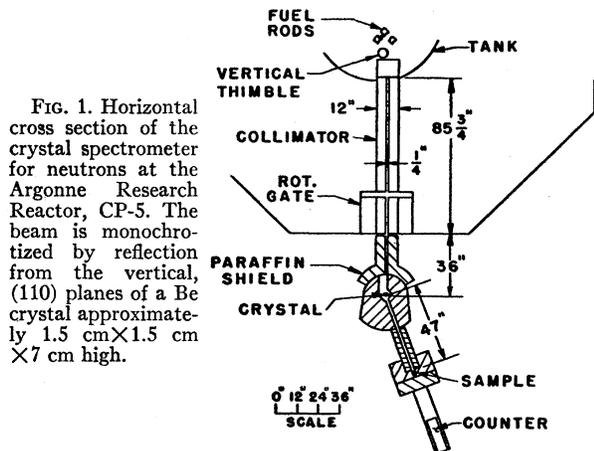
FIG. 1. Horizontal cross section of the crystal spectrometer for neutrons at the Argonne Research Reactor, CP-5. The beam is monochromatized by reflection from the vertical, (110) planes of a Be crystal approximately 1.5 cm  $\times$  1.5 cm  $\times$  7 cm high.
