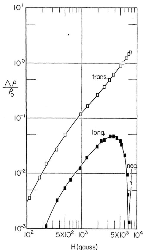
FIG. 5. Magnetoresistance at 78°K (sample 6).
