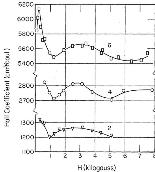
FIG. 7. Hall coefficient as a function of magnetic field strength at 78°K.
