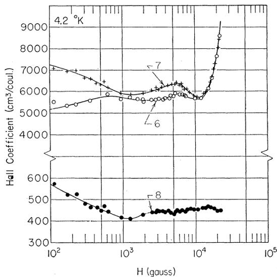
FIG. 11. Hall coefficient as a function of magnetic field strength at 4.2°K.
