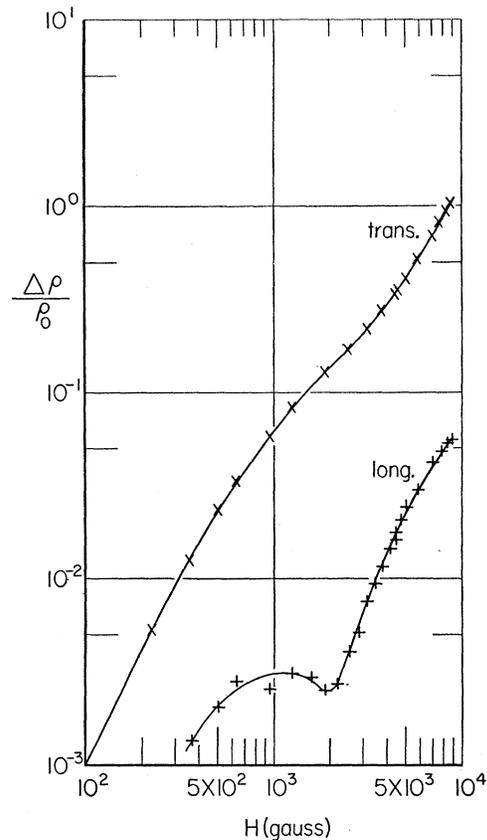
FIG. 3. Magnetoresistance at 78°K (sample 3).
