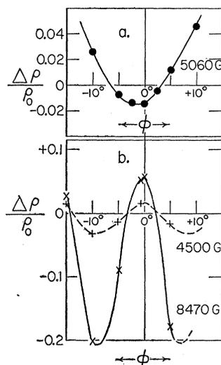
FIG. 2. Angular dependence of magnetoresistance, (a) for sample 4; (b) for sample 3. ( $\phi$  is the angle between  $I$  and  $H$ .)
