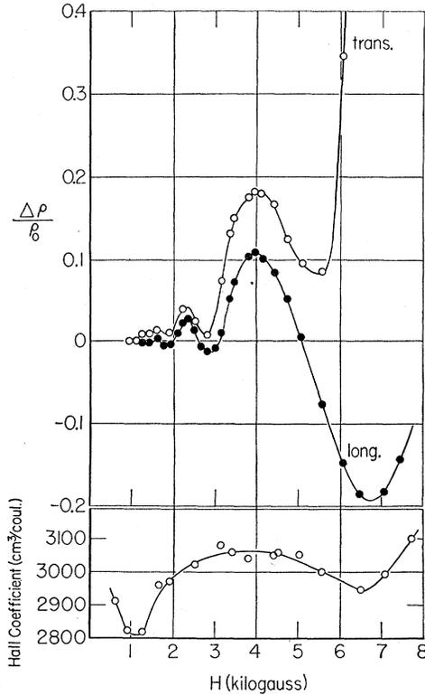
FIG. 9. Magnetoresistance and Hall coefficient at 1.7°K (sample 4).
