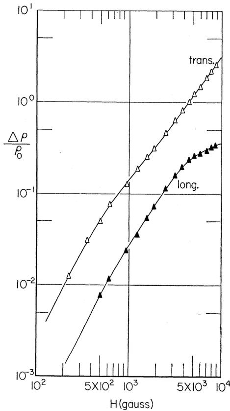
FIG. 6. Magnetoresistance at 78°K (sample 7).
