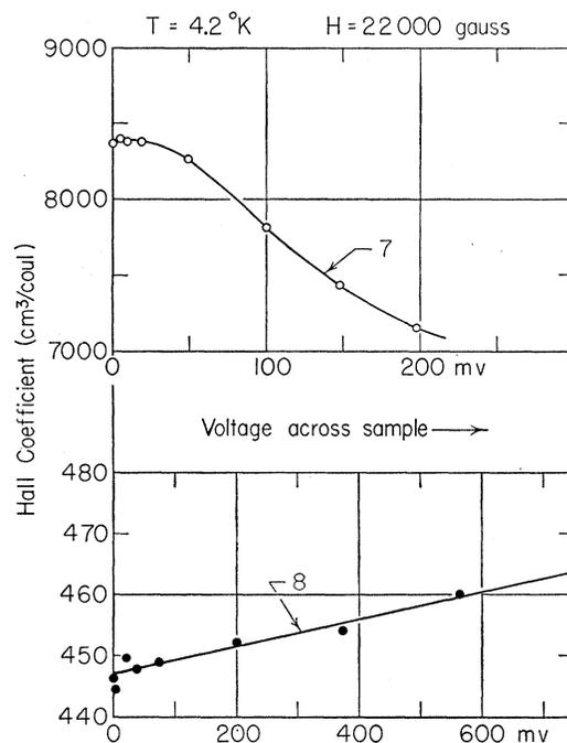
FIG. 12. Hall coefficient as a function of electric field strength.
