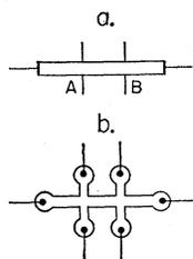
FIG. 1. Geometry of samples and probe configuration; (a) shape of samples 4-7; (b) shape of samples 1-3.
