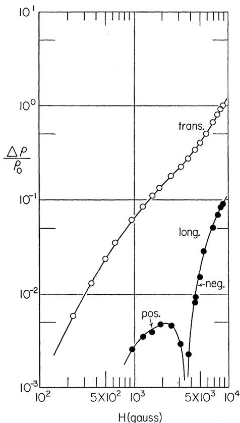
FIG. 4. Magnetoresistance at 78°K (sample 4).
