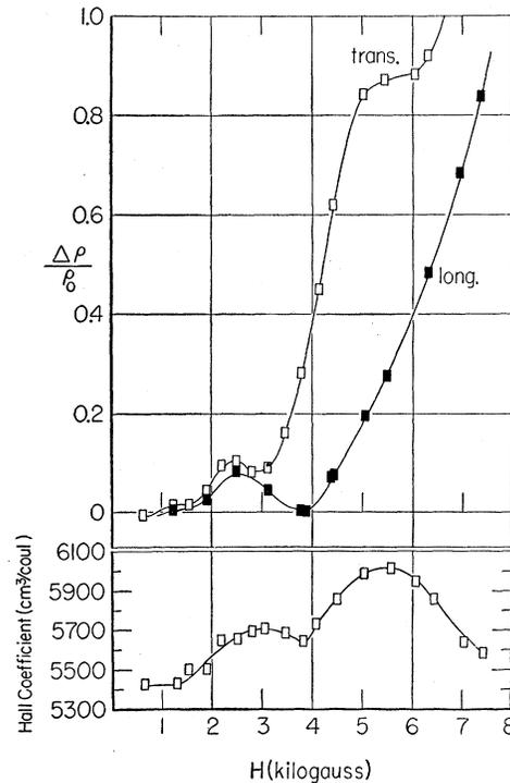
Fig. 8. Magnetoresistance and Hall coefficient at 1.7°K (sample 6).
