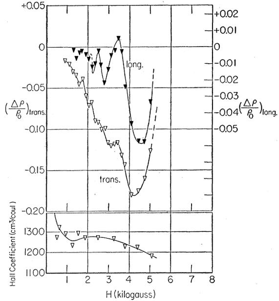
FIG. 10. Magnetoresistance and Hall coefficient at 1.7°K (sample 2).
