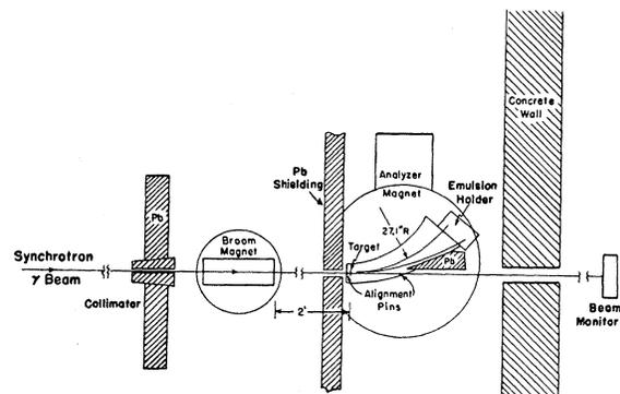
FIG. 1. Experimental arrangement for emulsion exposure shown in the median plane of the synchrotron.
