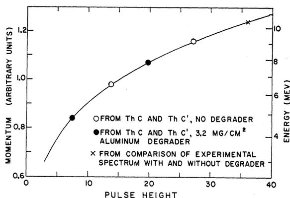
FIG. 3. Calibration curve of momentum and energy as a function of pulse height for alpha particles in the breakup detector. The curve includes a correction for the average energy loss in the (thick) target.
