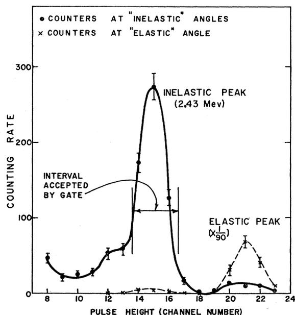
Fig. 2. Pulse-height distributions in the phoswich due to alpha particles scattered from beryllium. The alpha particles are observed in coincidence with particles in the breakup detector.
