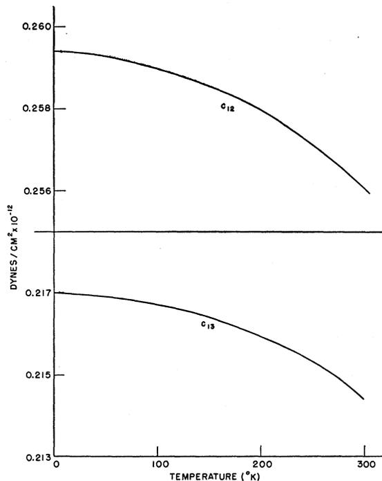
FIG. 3. The adiabatic elastic constants  $c_{12}$  and  $c_{13}$  versus temperature. These quantities are not obtained directly from a single velocity measurement.
