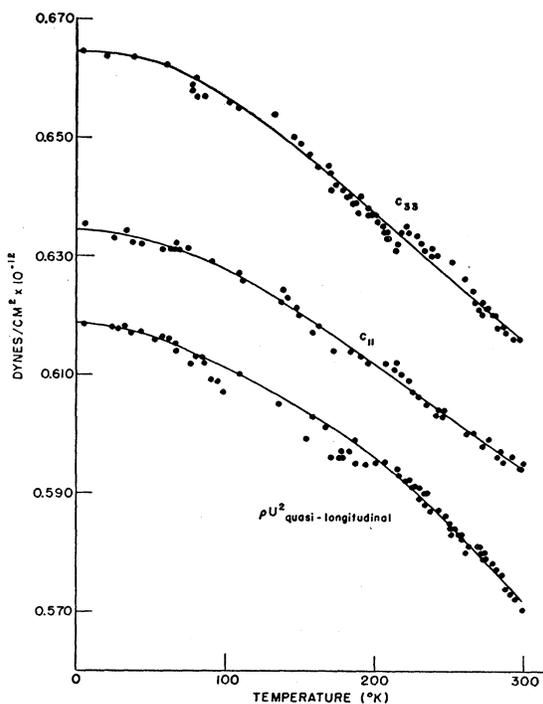
FIG. 2. The adiabatic elastic constants  $c_{11}$  and  $c_{33}$  and  $\rho U^2$  for the quasi-longitudinal wave in the direction at  $45^\circ$  to the  $c$  axis versus temperature.
