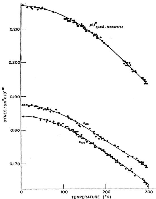
FIG. 1. The adiabatic elastic constants  $c_{44}$  and  $c_{66}$  and  $\rho U^2$  for the quasi-transverse wave in the direction at  $45^\circ$  to the  $c$  axis versus temperature.
