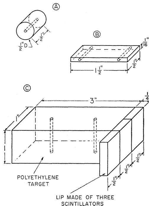
FIG. 2. Targets; (a) is of carbon or polyethylene and is dropped on a single nylon thread; (b) and (c) are of polyethylene and require two threads for orientation. The lip and front surface of (c) are scintillators made of terphenyl-loaded polystyrene.
