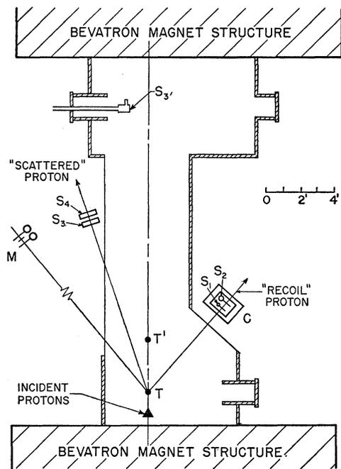
FIG. 1. Experimental arrangement.  $T$  and  $T'$  are alternate target locations;  $S_1$  and  $S_2$  are inside-radius scintillation counters on remote-controlled cart  $C$ ;  $S_3$  and  $S_4$  are outside-radius scintillation counters;  $S_3'$  is alternate outside counter, which can be rotated.
