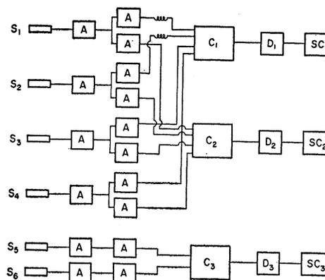
FIG. 3. Block diagram of electronics.  $S_1, \dots, S_6$  are scintillation counters.  $C_1$  and  $C_2$  are identical fast-coincidence circuits;  $D_1, D_2$ , and  $D_3$  are fast discriminators.  $C_3$  is the coincidence circuit for the monitor telescope. The  $A$ 's are Hewlett-Packard 460-A distributed amplifiers.  $SC_1, SC_2$ , and  $SC_3$  are scalars.
