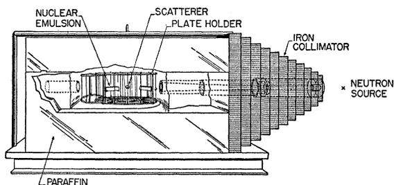
FIG. 1. Experimental arrangement for measuring angular distributions.
