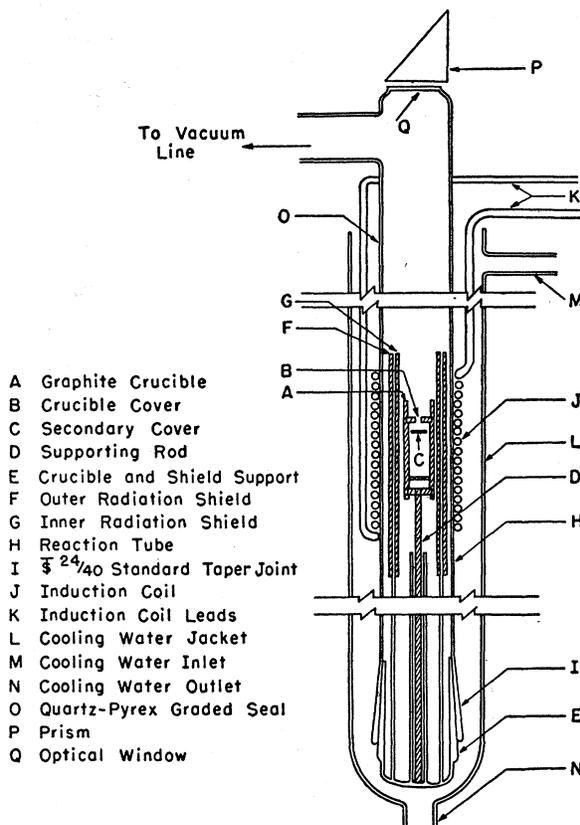
FIG. 3. Diffusion apparatus for the constant-surface-concentration experiments.
