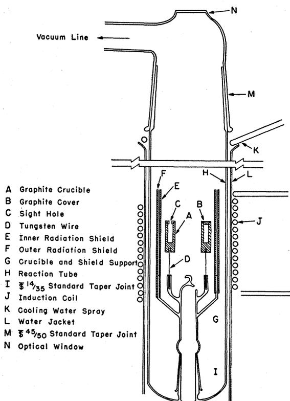
FIG. 2. Diffusion apparatus for the instantaneous-surface-source experiments.
