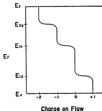
FIG. 2. The dependence of the charge on the flaw upon the Fermi level.
