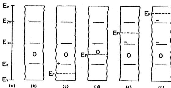
FIG. 1. Energy-level scheme for a flaw with possible charge conditions 1, 0, -1, and -2. (a) The energy levels and their notation; (b) the energy band diagram; (c)-(f) the dependence of charge condition upon the Fermi level. [To be consistent with the text,  $E_d$  should be replaced by  $E_{1d}$  in (a).]
