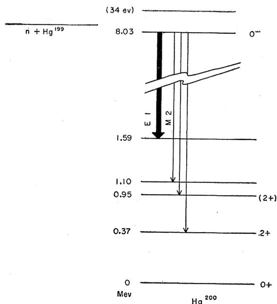
FIG. 1. Schematic diagram of the level structure of  $\text{Hg}^{200}$  as reported by Adyasevich *et al.* in reference 4.
