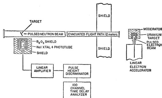
FIG. 2. Schematic diagram of the experimental apparatus associated with the neutron capture gamma-ray observation.
