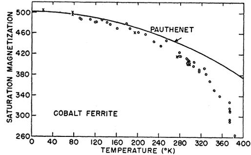
FIG. 4. Magnetic moment (*M*) as a function of temperature for cobalt ferrite.
