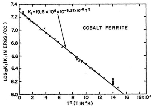
FIG. 3. Log<sub>10</sub>K<sub>1</sub> as a function of T<sup>2</sup> for cobalt ferrite.
