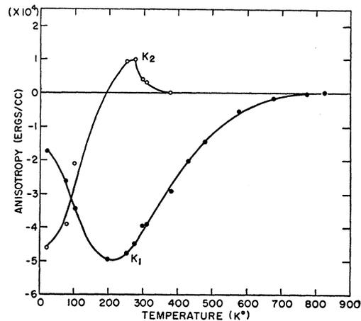
FIG. 5. First (*K*<sub>1</sub>) and second (*K*<sub>2</sub>) anisotropy constants of nickel cobalt ferrite as a function of temperature.
