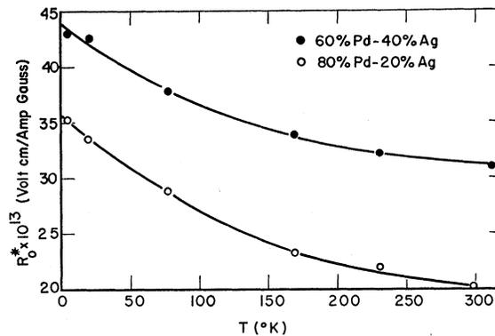
FIG. 3. Hall coefficient versus temperature for the two Pd-Ag alloys.
