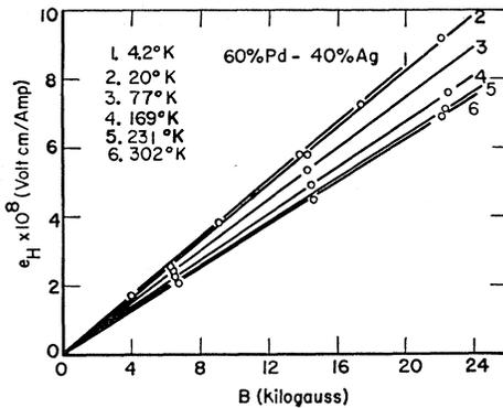
FIG. 1. Hall electric field per unit primary current density versus magnetic induction for 60% Pd-40% Ag at various temperatures.
