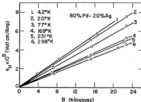
FIG. 2. Hall electric field per unit primary current density versus magnetic induction for 80% Pd-20% Ag at various temperatures.
