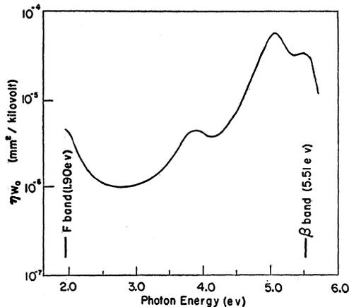
FIG. 7.  $\eta w_0$  versus photon energy in KI at 80°K.
