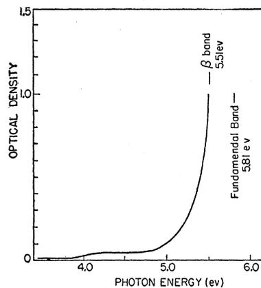
FIG. 8. Optical absorption of "pure" KI at 80°K.
