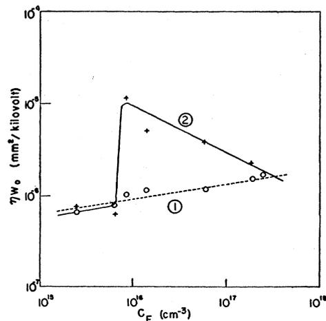
FIG. 6.  $\eta w_0$  versus  $c_F$  in KBr at  $80^\circ\text{K}$ . Curve 1, photon energy = 4.20 electron volts. Curve 2, photon energy = 5.50 electron volts.
