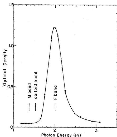
FIG. 1. The *F* band in KBr at room temperature. Crystal thickness 0.71 mm;  $c_F = 1.6 \times 10^{17} \text{ cm}^{-3}$ . The accepted locations of the *F*, *M*, and colloid bands are indicated.
