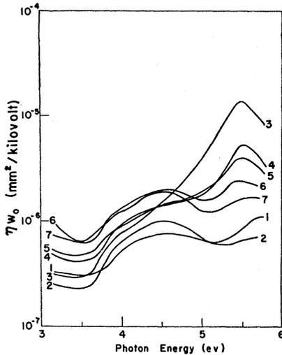
FIG. 5.  $\eta w_0$  versus photon energy in KBr at  $80^\circ\text{K}$ . See Table I for data pertaining to each curve.
