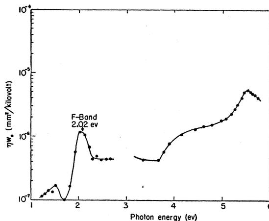
Fig. 4.  $\eta w_0$  versus photon energy in KBr at 80°K. Low-energy data from crystal 1.29 mm thick with  $c_F = 1.49 \times 10^{16}$  cm<sup>-3</sup>. High-energy data from crystal 1.23 mm thick with  $c_F = 1.42 \times 10^{16}$  cm<sup>-3</sup>.
