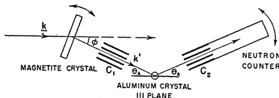
FIG. 1. Schematic drawing of the apparatus. The  $01\bar{1}$  axis of the magnetite crystal is normal to the plane of the spectrometers.
