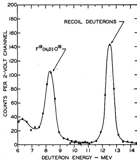
Fig. 1. Energy spectrum of forward  $D(n,n)D$  elastic-recoil deuterons and deuterons emitted in the forward direction from the  $F^{19}(n,d)O^{18}$  ground-state reaction.
