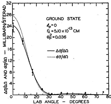
FIG. 3. Experimental and normalized theoretical differential cross sections for the ground-state F<sup>19</sup>(n, d)O<sup>18</sup> reaction. The solid curve has been corrected for the effect of the finite aperture of the detector.
