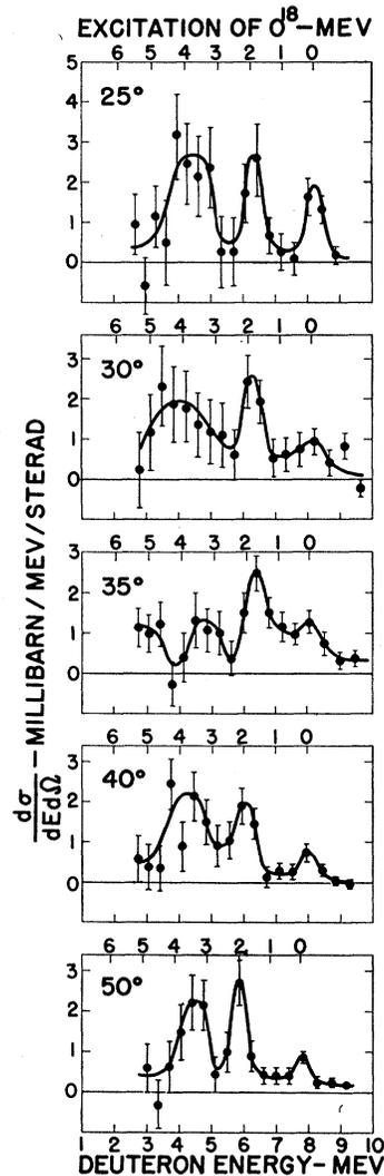
Fig. 2. Energy spectra of deuterons emitted in various directions from the  $F^{19}(n,d)O^{18}$  reactions.
