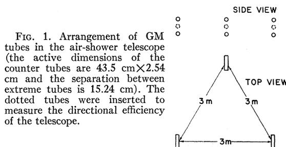
FIG. 1. Arrangement of GM tubes in the air-shower telescope (the active dimensions of the counter tubes are  $43.5 \text{ cm} \times 2.54 \text{ cm}$  and the separation between extreme tubes is  $15.24 \text{ cm}$ ). The dotted tubes were inserted to measure the directional efficiency of the telescope.
