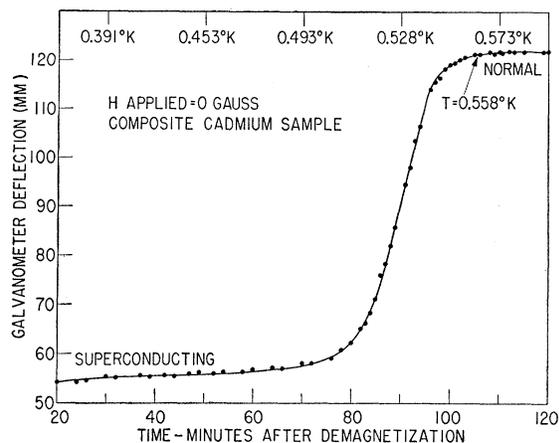
FIG. 7. The galvanometer deflection obtained in zero applied magnetic field for the composite cadmium sample as a function of the time after demagnetization.
