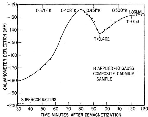
FIG. 8. The galvanometer deflection obtained in an applied magnetic field of 10 gauss for the composite cadmium sample as a function of the time after demagnetization.
