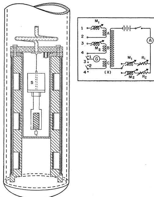
FIG. 1. Schematic diagram of the lower Dewar assembly.
