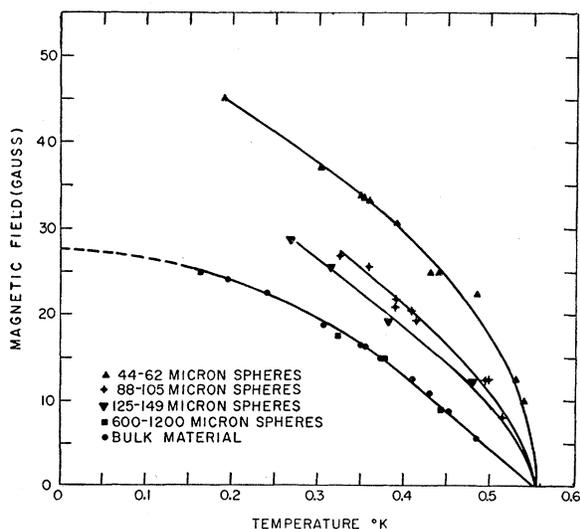
FIG. 2. The critical magnetic fields of all the specimens as a function of the absolute temperature.
