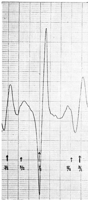
FIG. 2. Typical spectrum of the pentad m = -5/2 . The transitions from left to right are M = 3/2 \rightarrow 1/2 , M = -5/2 \rightarrow -3/2 , M = 1/2 \rightarrow -1/2 , M = 5/2 \rightarrow 3/2 , and M = -3/2 \rightarrow -1/2 .
